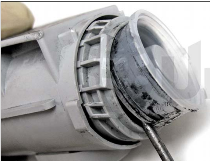
6. Carefully lift the toner fill plug out as shown. Be careful not to damage the plastic housing.
