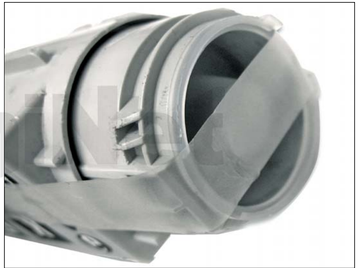
18. Wrap the remaining seal around the toner fill plug as shown.
