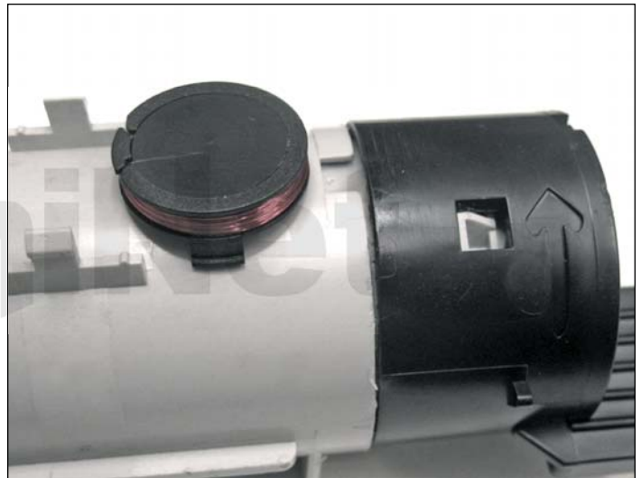
26. Place the new contact chip on the cartridge as shown.
