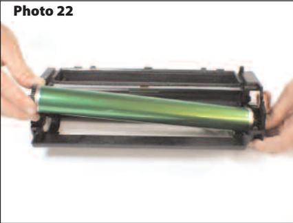
**NOTE:** If the drum being used is damaged and the axle cannot be removed from the drum by simply pulling the axle out, remove the small gear from the end of the drum. Install the drum axle into the new drum and glue the gear into place.
