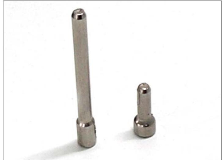
8. Notice the sizes of the pins for the contact side (short) and the gear side (long).
