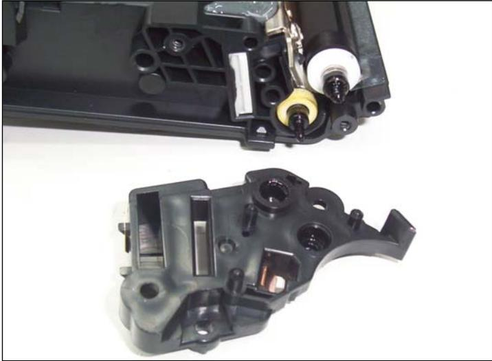
24. Slide off the gearless support plate.
