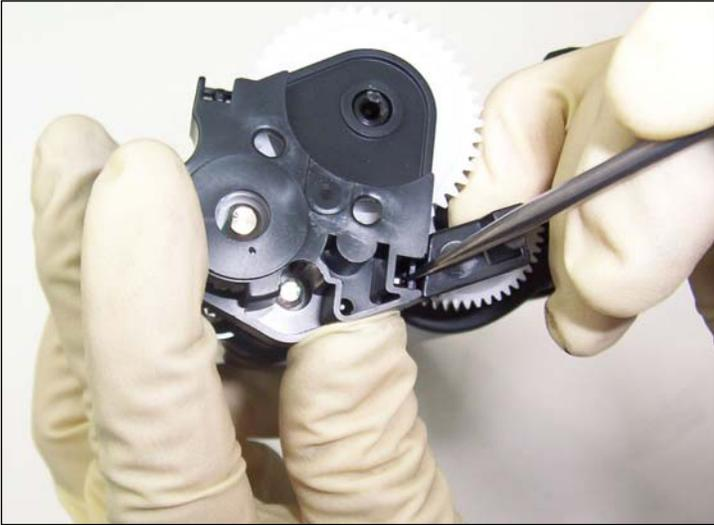
16. Locate the third tab holder shown near the bottom.
