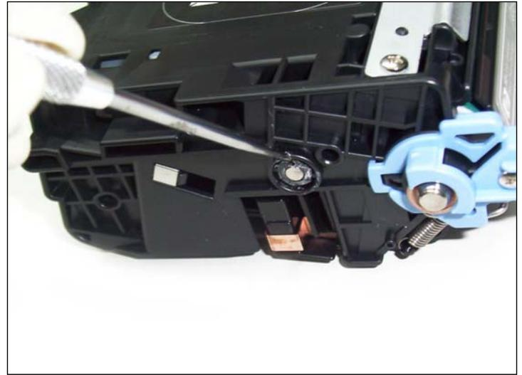
4. Insert a scribe or pin pusher through the hole to pull the pin out on one side.
