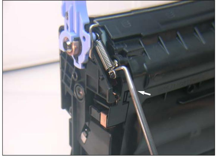
10. Release the spring on the gearless side.
