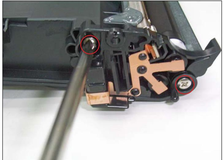
**REMOVING THE GEARLESS SUPPORT PLATE**
