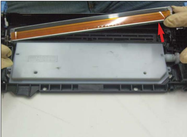
42. Now slowly but firmly, pull the loose end of the wiper blade upward with your hand as shown until it is completely removed.
