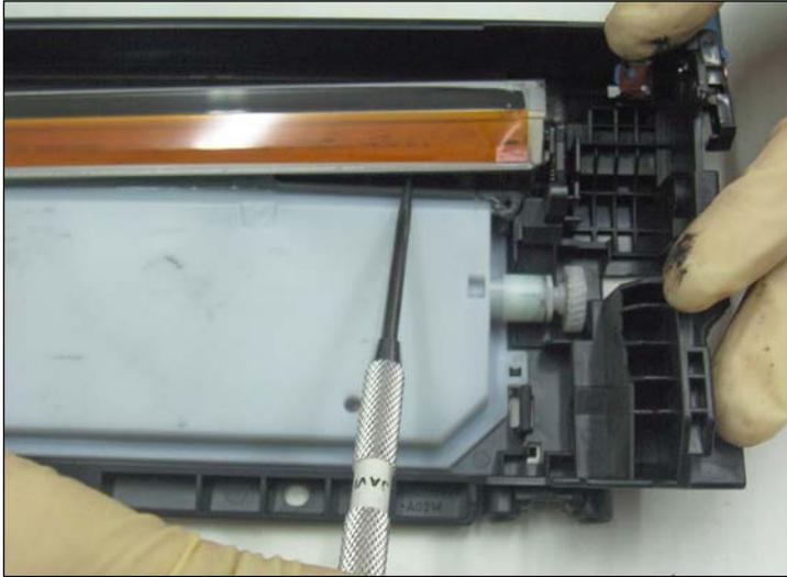
40. Wedge a small scribe or small screwdriver between the base of the wiper blade and the hopper beneath that it adheres to.
