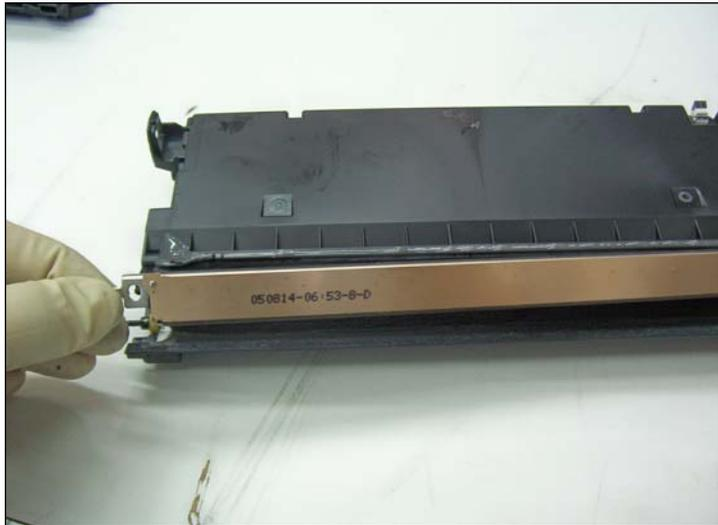
28. Once the blade has been separated far enough from the hopper, continue to pull it completely out from one side using your hand.
