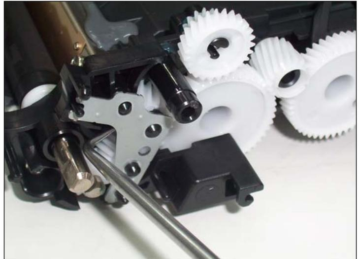
19. Using a hook tool, slide out the gear retaining plate. This will reveal three remaining drive gears beneath.
