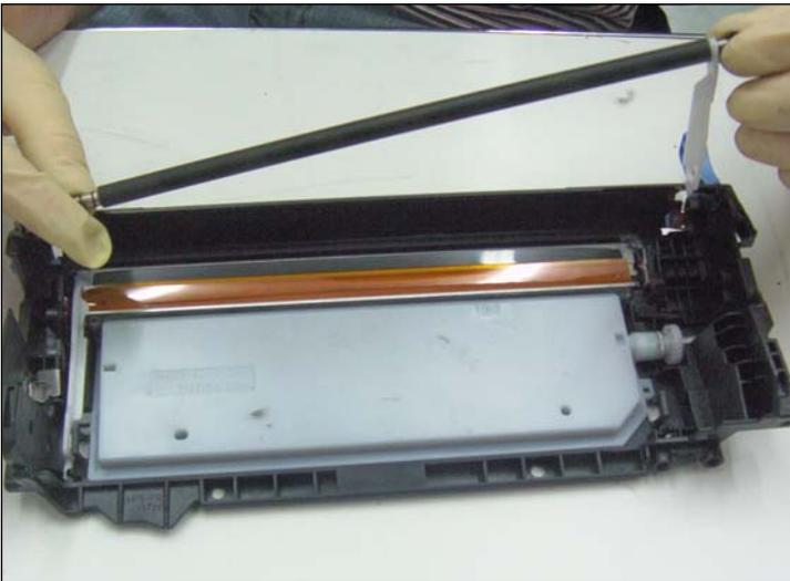
38. After releasing both arms, remove the PCR.
