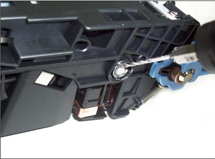
3. Drill a small hole just above the pin on both sides of the cartridge.
