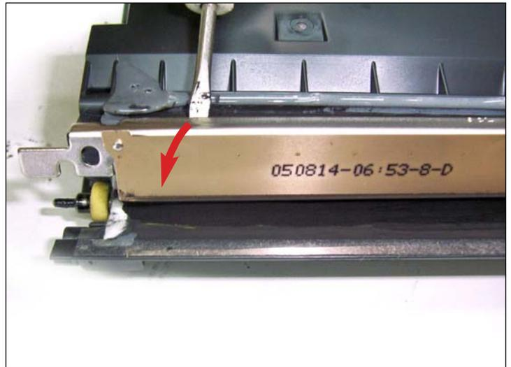
27. Using a small flathead screwdriver, pry the blade far enough to separate it from OEM adhesive.
