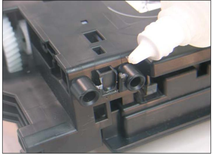
48. Apply a small amount of plastic cement into the plastic slots. This will seal the replacement chip into place from each side.
