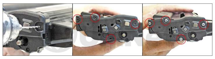
33 Drill four small holes that correspond to the screw size your using.
