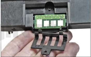
38. To replace the chip, slice the top of the plastic rivet off with the chisel blade knife.
