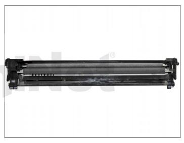
18. Place a small amount of conductive grease in the holders, and install the PCR.
