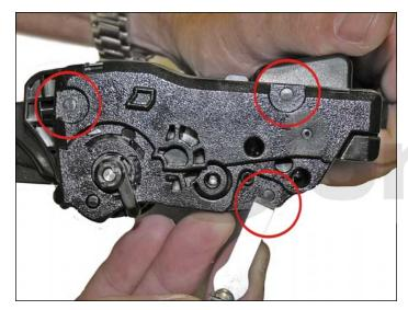
1. Place the cartridge with the handle up, facing towards you. With the chisel blade knife, slice off the heads of the three plastic rivets. Leave the end cap in place for now.
