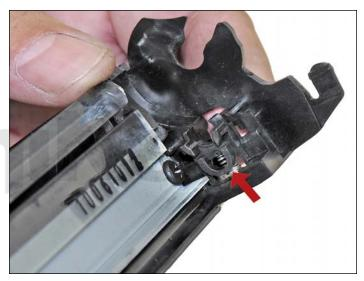
12. Remove both the PCR holders by pressing in on the tabs at the bottom of the holder. These holders need to be removed to allow access to the wiper blade.
