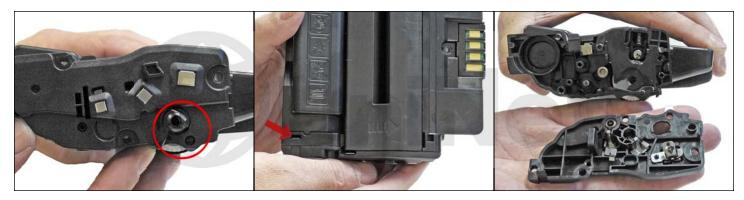
6. On the right side end cap, remove the remaining arm and press in on the top tab and remove the end cap.
