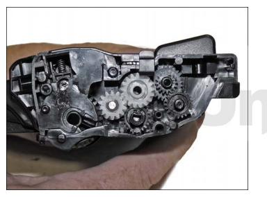
5. Remove the gears.
