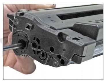
3. Remove the drum axle arm from the right or large gear side of the cartridge.
