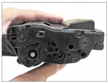
35. Clean the hubs on the gear side end cap, and replace the conductive grease.
