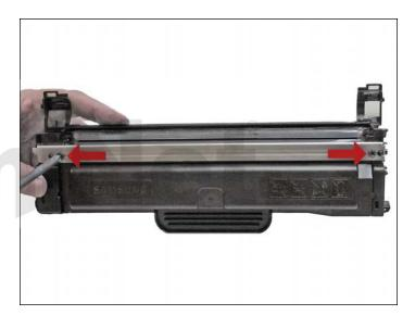
26. Install the doctor blade and two screws.
