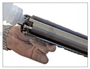
28. Fill the hopper with toner for use in Dell 1130, replace the fill plug, and check for leaks.
