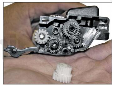
29. Install the gears as shown.
