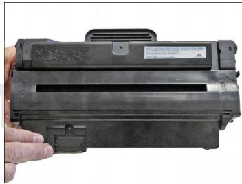
31. Slide the middle top cover/PCR assembly into place.
