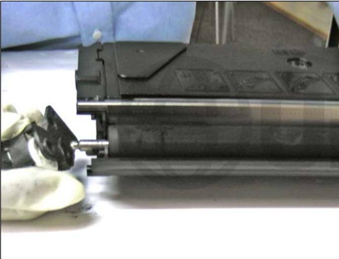
7. Gearless side developer roller support removed.
