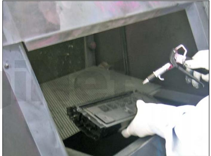
20. Clean the cartridge thoroughly using compressed air or vacuum. Refill with 245 grams of M20 toner and reassemble following the preceding steps in reverse. Before re-installing the gearside end cap a new smartchip must be fitted.
