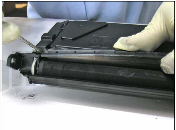
4. Using a flat screwdriver, pry loose the doctor blade cover from either side of the toner cartridge as shown.
