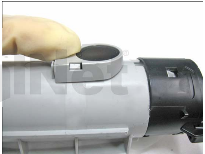
28. Press down until the tabs lock in place.
