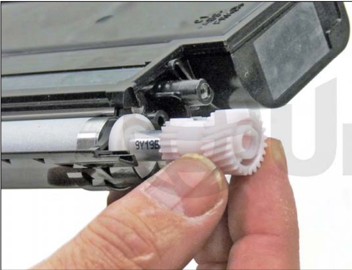
9. Remove the large magnetic roller drive gear.
