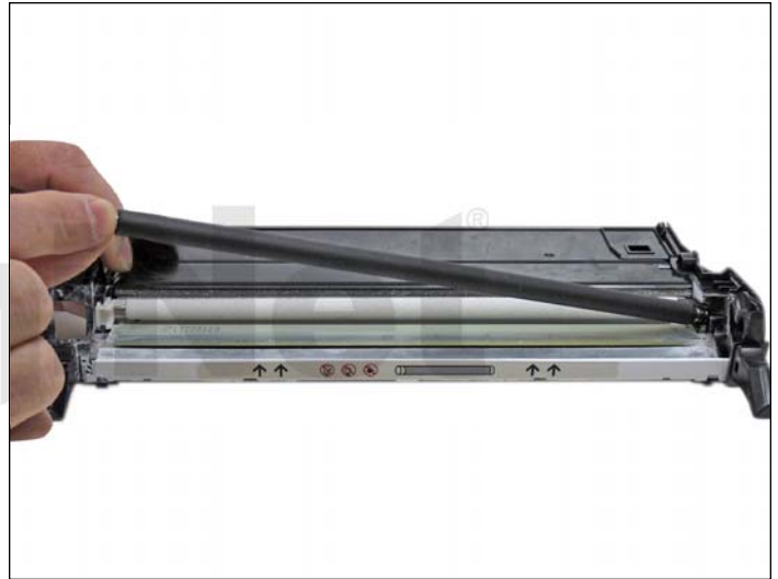
26. Remove the PCR and clean with a lint free cloth.
