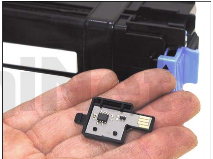
10. Slide the holder out of the cartridge and replace the chip.
