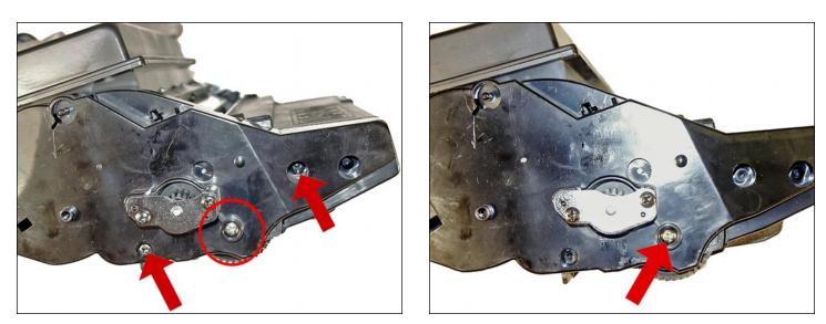
6. Remove the two black screws from the right side end cap.
