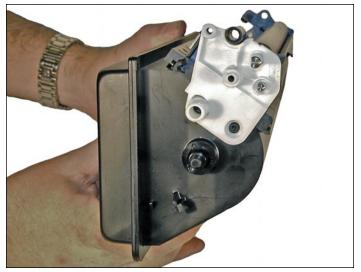
44. Install the white plastic alignment plate on the gear side.
