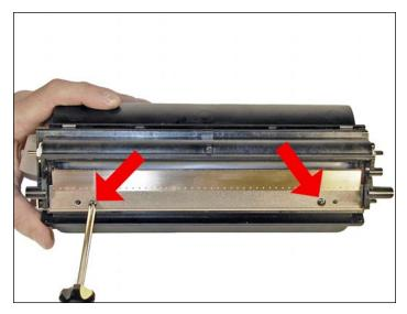
41. Clean or replace the doctor blade. Install with the two screws into the hopper.
