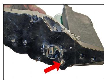
12. On the waste hopper, remove the gold colored screw from the drum axle; work the waste section away from the frame.
