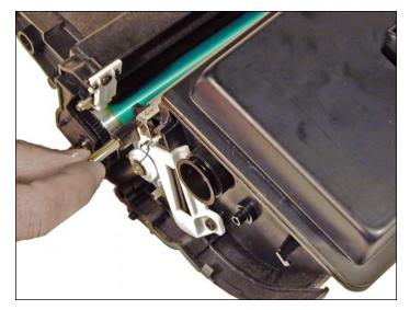
10. Slide the metal rod located above the developer roller away from the remaining end cap to free it from the end caps.
