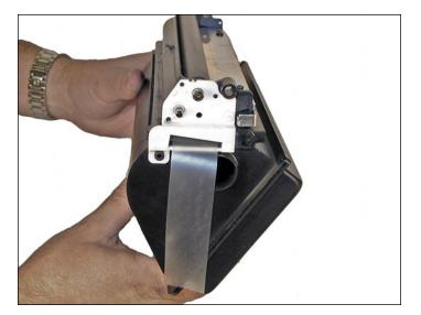
43. Install the white plastic alignment plate and the screw on the fill plug side.
