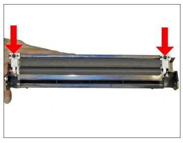
16. Remove the two screws on the PCR assembly.
