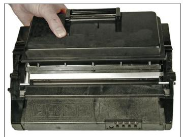
62. Align and snap the end cap into place.
