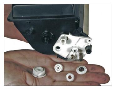
29. Remove the remaining three gears and the bearing.
