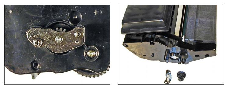
7. Remove the two screws from the metal plate.
