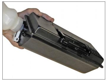
52. Fill the hopper with toner for use in the Phaser 3500 (350g for the 12k, 175g for the 6k). Replace the fill plug, and check for leaks.
