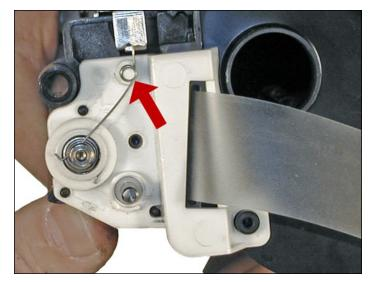
46. Install the small spring as shown onto the developer roller shaft.
