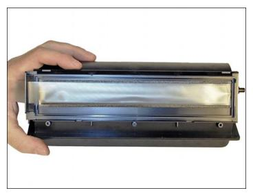
39. Install the seal fold over the pull-tab so it sits over the foam edge seal. Slide the tab through the slot.
