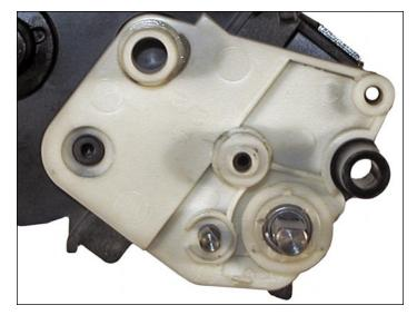
47. Install the bearing onto the developer roller shaft, gear side of the hopper.
