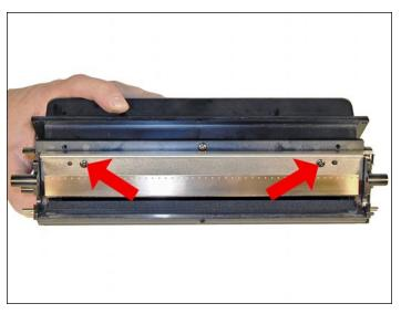
36. Remove the two screws and the doctor blade.
