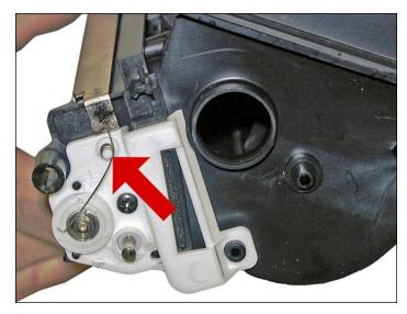
32. On the opposite side of the hopper, release and remove the small spring.
