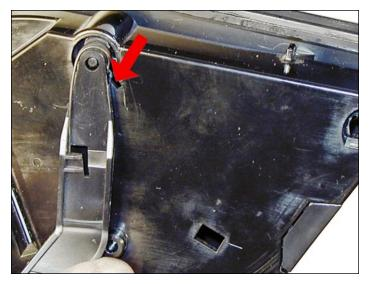
66. Install the drum-cover arms. Place the arm into place, and rotate the tail of the springs so they fit into their respective slots.
