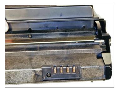
68. Remove the screw and cover for the chip. Replace the chip. Make sure you match the chip to the toner load (high yield or low yield)!
