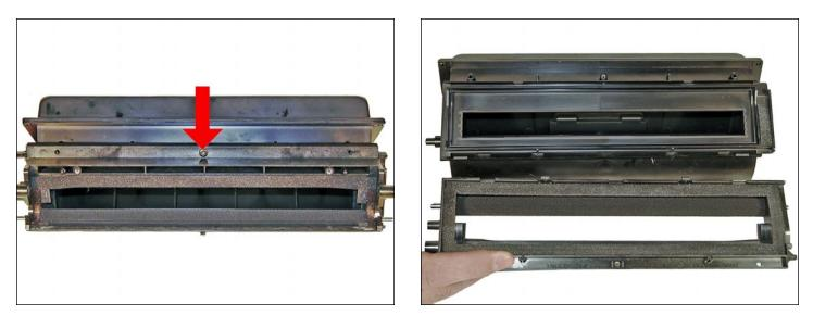
37. Remove the center screw from the toner hopper.
