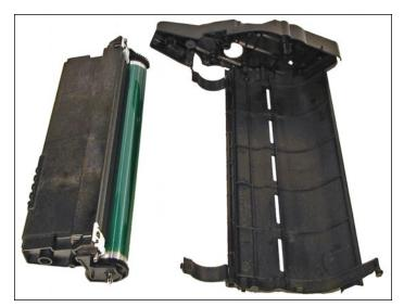
13. Remove the waste section from the frame.
