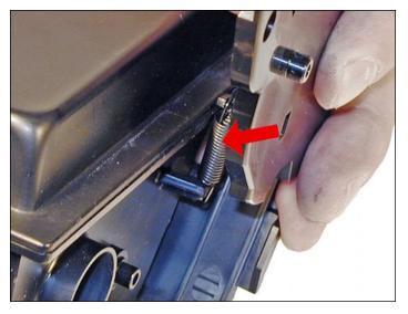
60. Install the spring from the end cap to the hopper.
