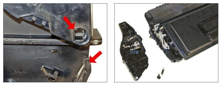
9. Carefully rock the left side end cap until it comes free from the cartridge frame. Turn the back edge up so it comes free from the hopper. The spring, and possibly a small gear, will fall from the cartridge. The installation of both parts will be shown later.
