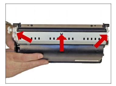
51. Install the bottom metal plate. Insert the three tabs first and rotate into place. Make sure all three locks (two sides and middle) snap into place!
