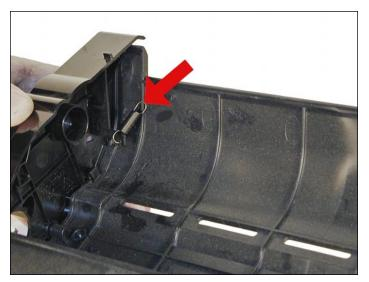
56. Install the hopper spring onto the end cap.
