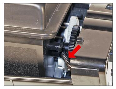
57. Place the hopper partially into the frame, and hook the spring onto the hopper.
