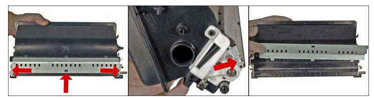
30. Remove the bottom metal plate.
