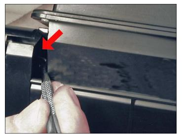
8. Using a spring hook, remove the two springs from the back of the toner hopper (one on the left, and one on the right side, about 1 inch from the back edge.
