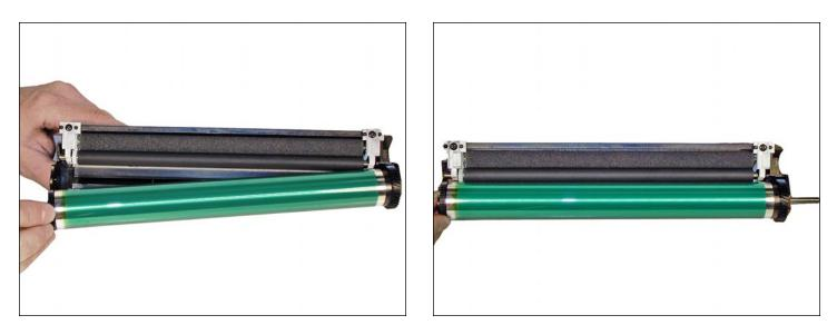
23. Install the drum, and drum axle (large gear to the non-gear side of the PCR).
