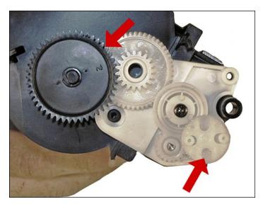
50. Install the large black gear, and the small white drive gear.
