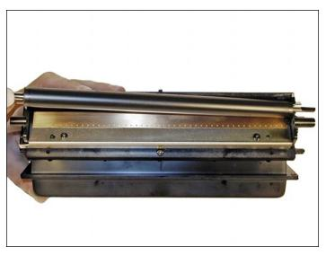
42. Install the developer roller, long shaft side to the gear side of the hopper (NON-fill plug side).
