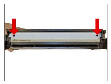
18. Remove the two screws on the wiper blade.
