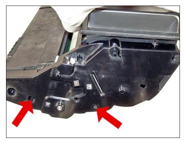
65. Install the two screws into the right side end cap.
