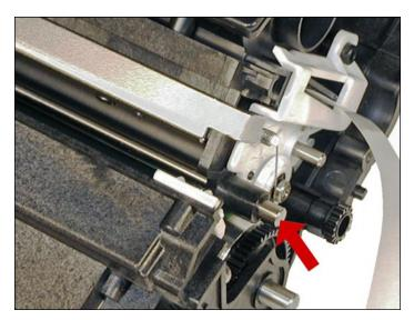
58. Partially install the metal rod on the toner hopper. Seat the hopper into the end cap, and seal the metal rod. Make sure the rod is seated into its hole, and the white drive gear is centered into the 1-inch hole.
