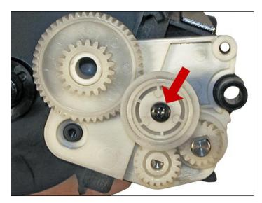
49. Install the center white gear and screw.
