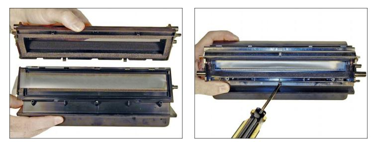
40. Slide the seal tab out the slot of the top cover. Set the three plastic tabs into their slots, and rotate the top cover down into place. Install the screw. Make sure the cover locks into place! Check the seam on the end of the hopper to be sure.
