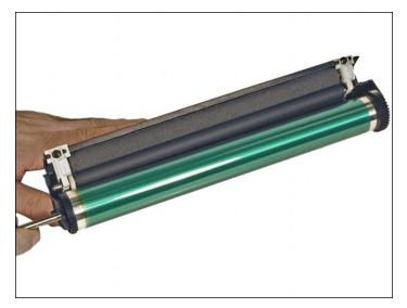
14. On the waste section, remove the drum axle by pulling it out from the small straight gear side.
