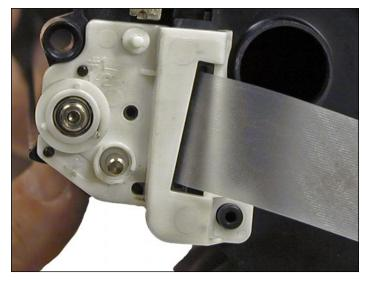
45. Install the bearing onto the developer roller shaft of the fill plug side.
