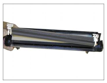
17. Pry up the white plastic holders, and remove the PCR assembly.
