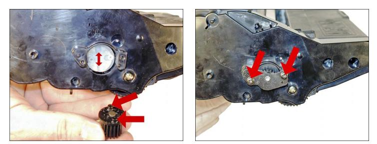
63. Install the drive gear, metal plate, and two screws.
