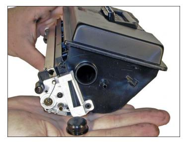
27. Remove the fill plug, and dump out all remaining toner from the hopper. Vacuum clean.
