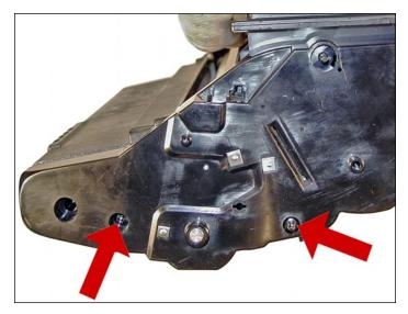
5. Remove the two screws on the left end cap.
