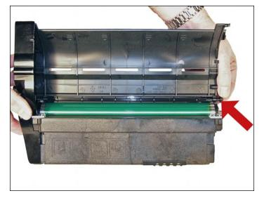
55. Make sure the small round black plastic rod is in place. Install the small drive gear (this is the gear that came loose when the end cap was removed).
