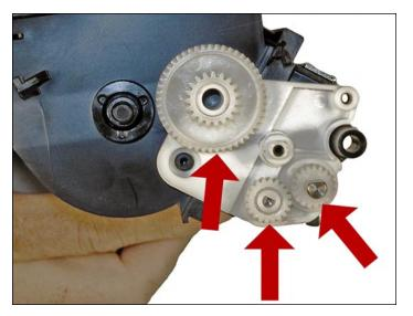
48. Install the three white gears as shown.
