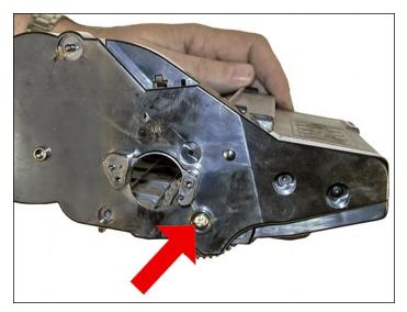
54. Install the gold screw into the drum axle.
