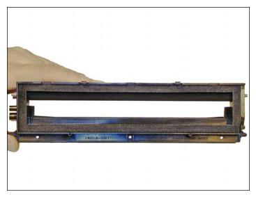
38. Clean out any remaining toner from both halves of the assembly. Make sure the foam seals are clean. If the supply roller is worn, it can easily be replaced now as well.
