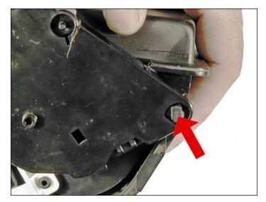
59. Rotate the remaining end cap and partially install it on the frame, so that the rear tab locks into place.
