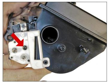
34. Remove the screw and the white plastic alignment plate.
