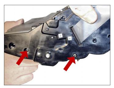
64. Install the two screws into the left side end cap.
