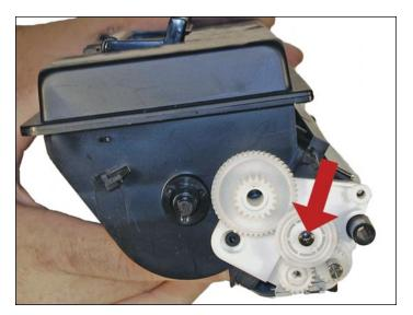
28. Remove the screw from the middle white gear.
