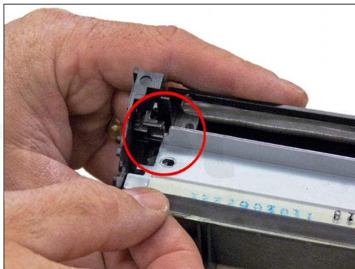
12. Remove the two screws from the wiper blade, and remove the blade
