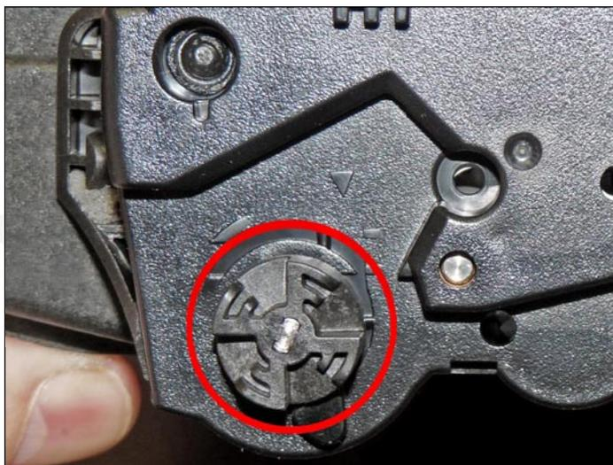
3. The drum axle arms on both sides of the cartridge stay with the end cap.
