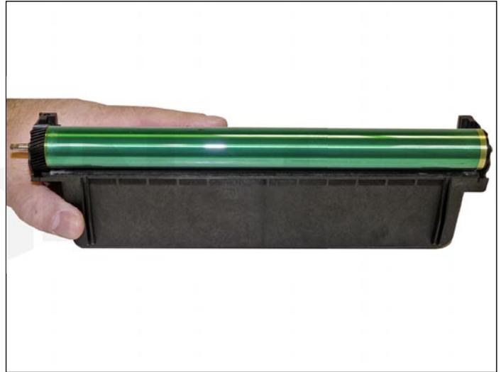
22. Install the drum, with the large gear to the gear (non-chip) side of the drum, into the waste hopper.
