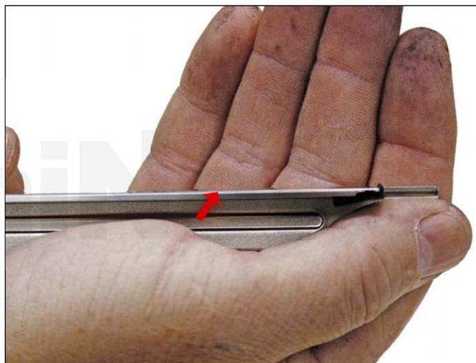
29. Make sure the doctor blade sealing foam and the developer roller seals are clean and intact.
