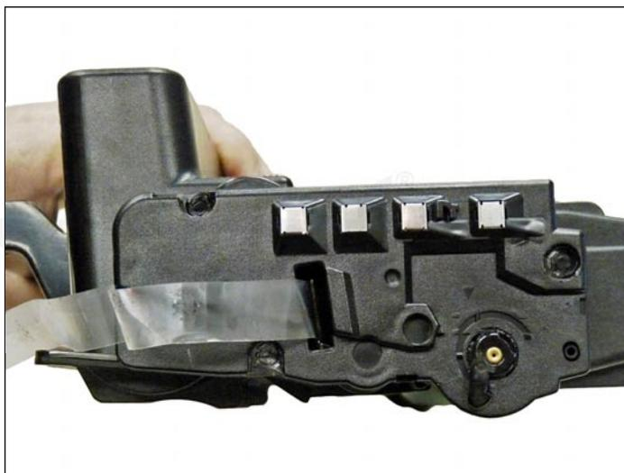
42. Clean the contacts on the left side end cap, and replace the conductive grease.
