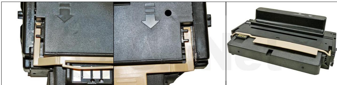
48. Install the protective cover around the cartridge.
