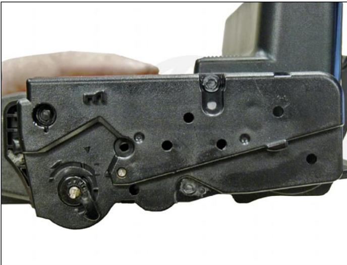
44. Clean the hubs on the gear or right side end cap.
