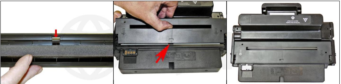
41. Slide the cleaned middle top cover/PCR cleaner assembly into place.
