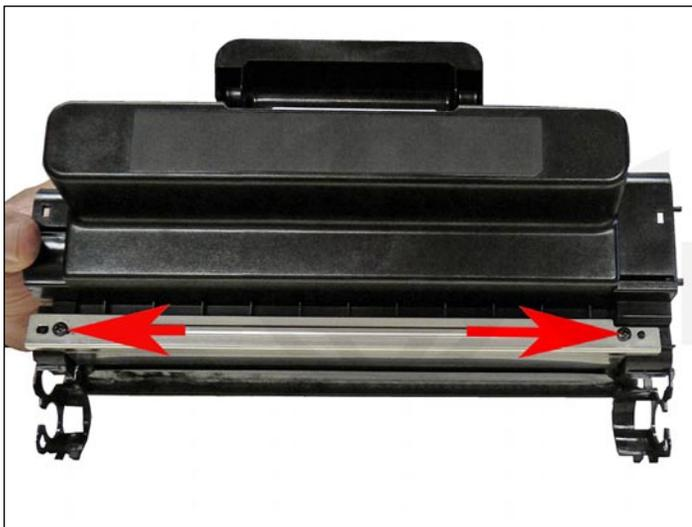
33. Install the doctor blade and two screws.
