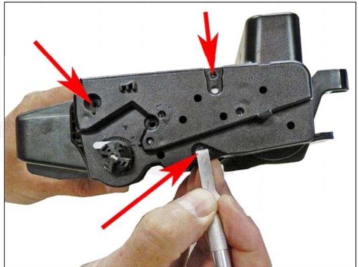
2. On the opposite side end cap, take the chisel blade knife and slice off the heads of the three plastic rivets. See Step 1 regarding recessed rivets. Leave the end cap on for now.
