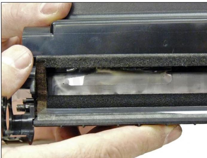
31. Install the seal (when available) through the developer roller opening.
