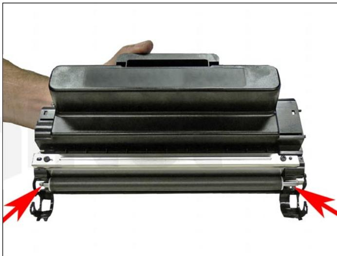
34. Clean the developer roller with a dedicated developer roller cleaner, and replace into the hopper.
