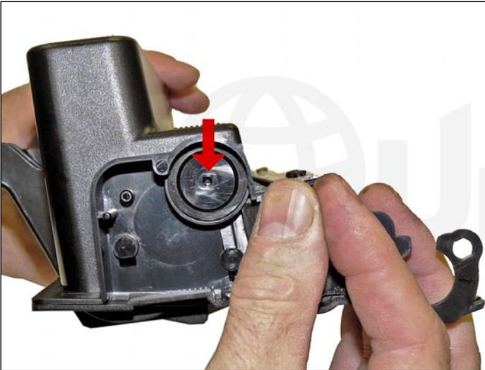
23. On the supply hopper, carefully pry out the fill plug and dump out any remaining toner. The fill plug can be difficult to remove as it is recessed. Take a small common screwdriver and work it around the edge lifting slightly until it comes loose.
