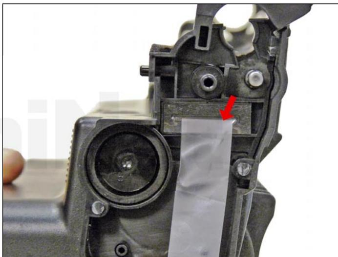
32. Pull the tail of the seal through the seal port.
