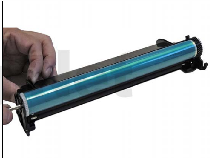
20. Install the drum and axle from the small gear side of the drum into the waste hopper. Make sure the keyed end of the shaft is on the small gear side.
