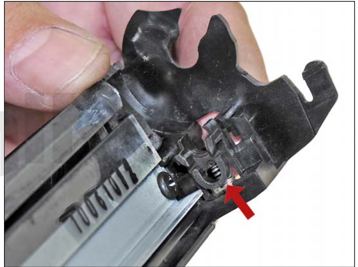
12. Remove both the PCR holders by pressing in on the tabs at the bottom of the holder. These holders need to be removed to allow access to the wiper blade.
