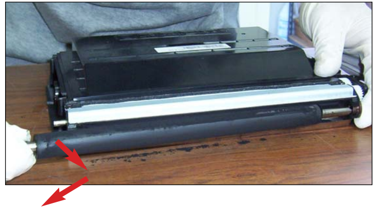
8. Slip the developer roller outward then slide it away toward the side of the cartridge.
