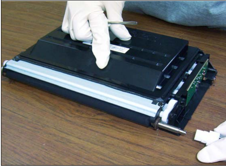
5. Remove the gears from each side. They should slip off fairly easily.
