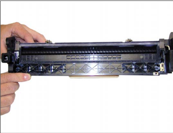
11. Clean out any toner from the hopper. Make sure you also clean out the auger post.
