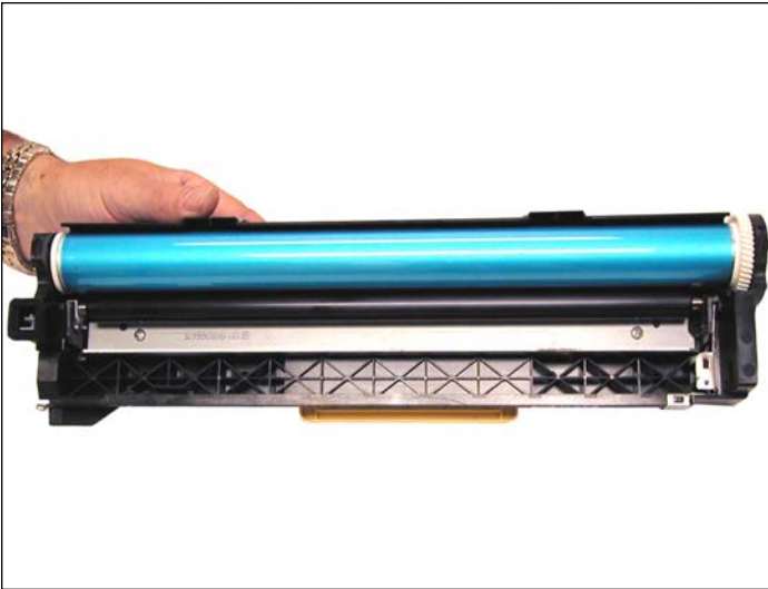
14. Place the drum in the hopper and carefully pace aside.
