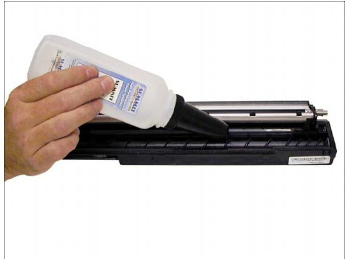
22. Pour in the new developer. Make sure you cover both augers.
