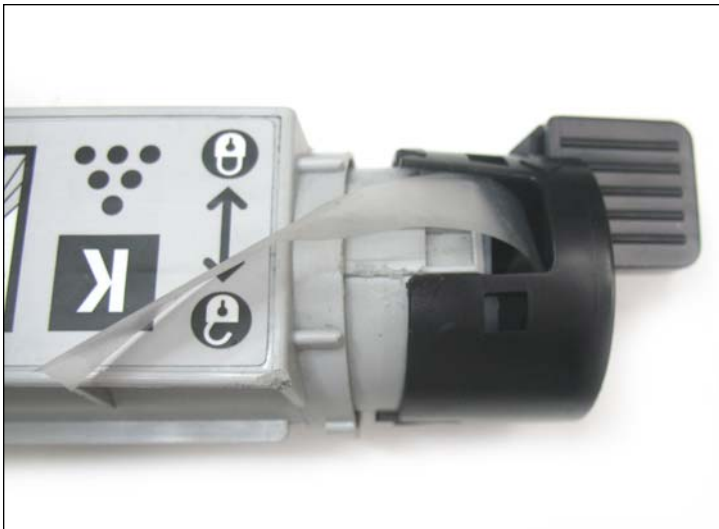
20. Place the gearless end cap, in its original positioning, over the seal and toner fill plug as shown.
