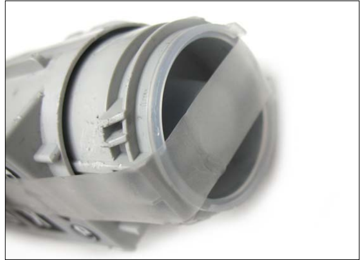
19. First, wrap the remaining seal around the toner fill plug as shown.
