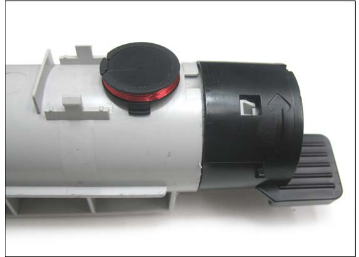
INSTALLING THE UNICHIP® CONTACT SMARTCHIP® 27. Place the new chip on the cartridge in the manner shown.
