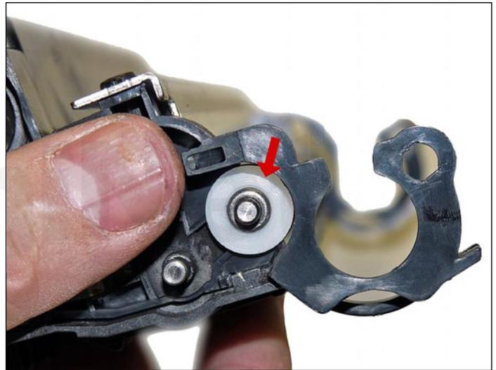
25. Remove the developer roller bushings from both sides.
