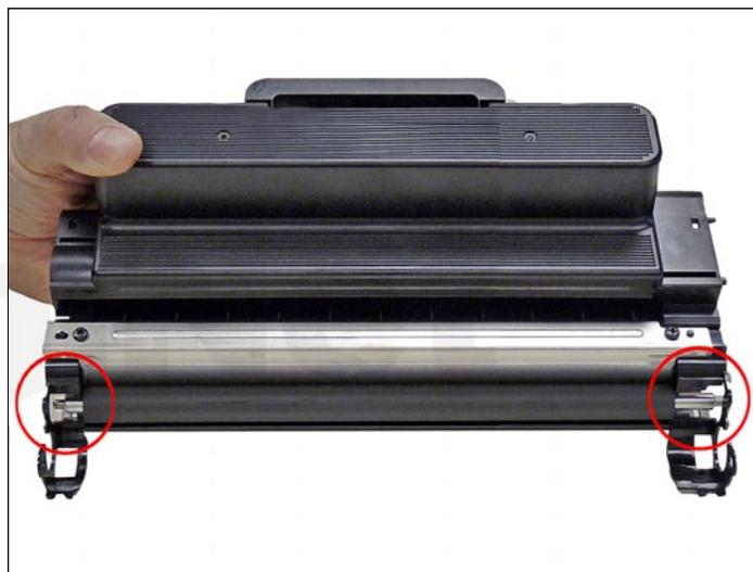
34. Clean the developer roller with a dedicated DVR cleaner, and replace into the hopper. Place the long shaft side to the gear side of the cartridge. It should snap in place if installed correctly.
