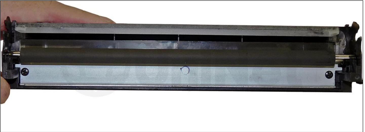
21. Place a small amount of conductive grease in the holders.
