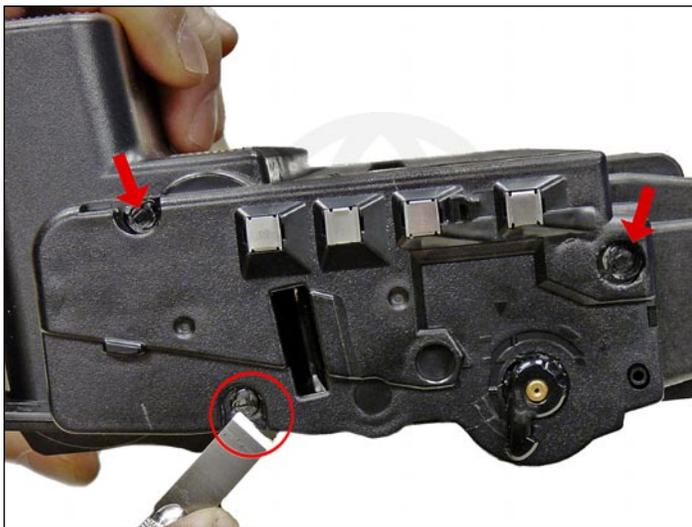
1. On the contact side of the cartridge, slice off the heads of the three plastic rivets with a chisel blade knife. If your knife is too wide, you may find it necessary to drill out the upper recessed rivets on both sides. Leave the end cap on for now.
