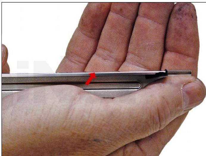
30. Clean the doctor blade edge, so there is no evidence of build up along the edge. If any buildup exists, the cartridge will streak. No chemicals should be used. We have found using a clean ice cream type wooden stick works great for scraping the blade clean without damaging it.
