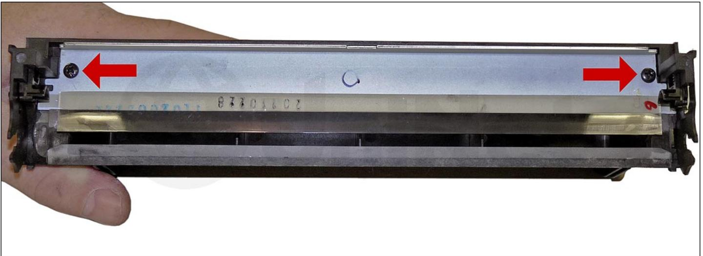
20. Install the new wiper blade and two screws.
