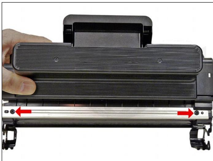
33. Install the doctor blade and two screws.
