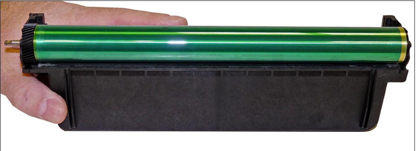
22. Install the drum with the large gear to the gear or non-chip side of the drum into the waste hopper.
