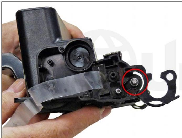
35. Clean and replace the conductive grease on the short shaft side of the roller.
