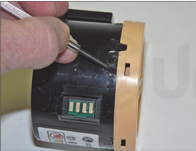
2. Gently pry up each tab until the top cover comes loose. Be careful here! The top cover can pop off and toner can go all over if you're not careful.
