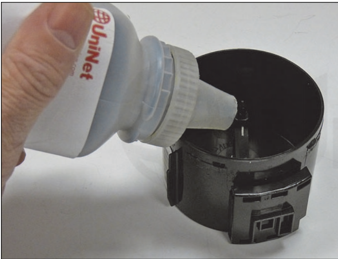
6. Clean out all the old toner from the cartridge and cover, fill with new toner.
