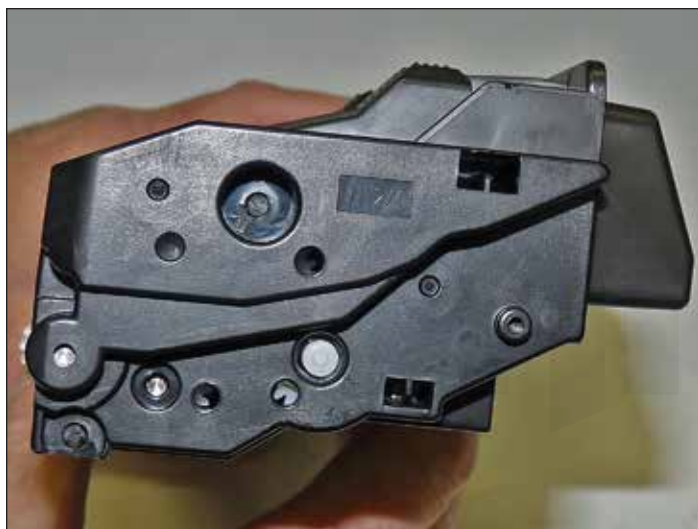
18. Install the gear side cover.
