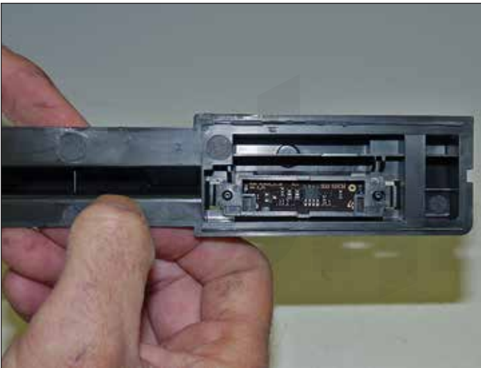
28. Install the chip holder back into the handle cover.
