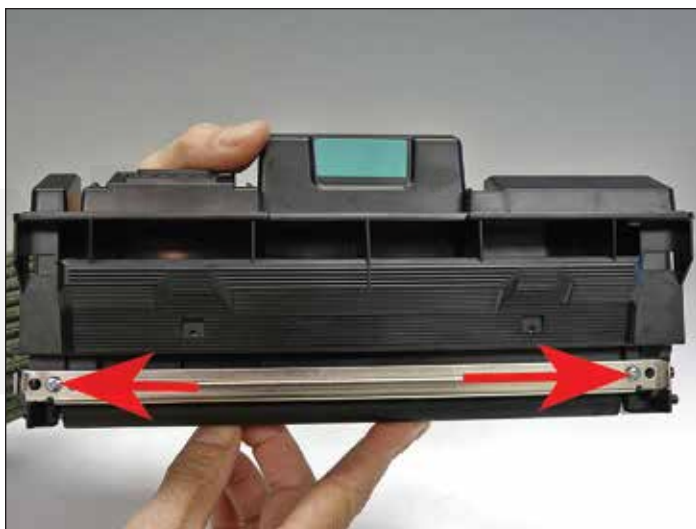
7. Remove the two screws on the doctor blade and remove the blade.
