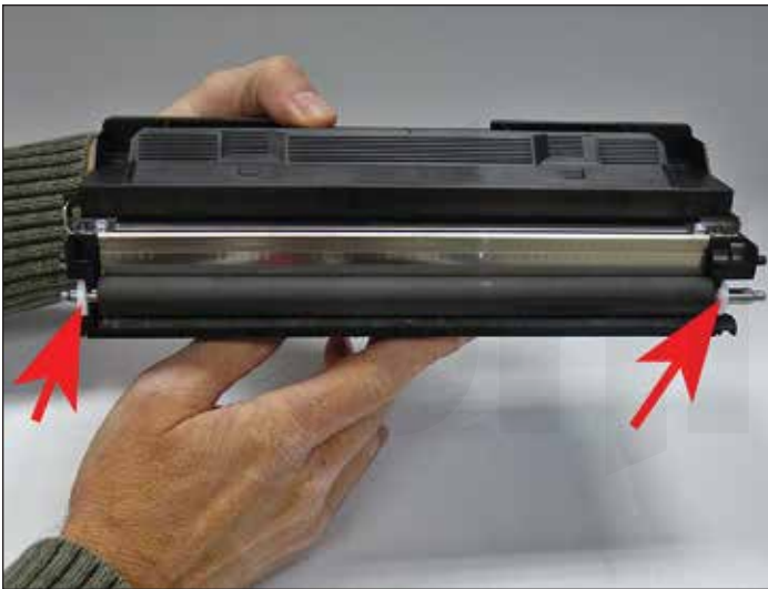
16. Install the two white developer roller washers.
