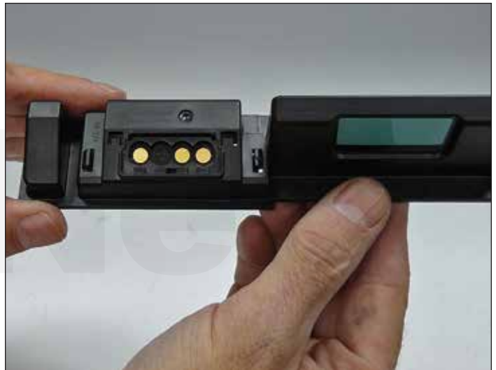
28. Install the chip holder back into the handle cover.
