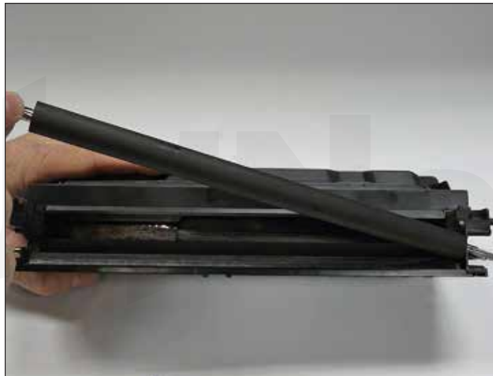
9. Remove the developer roller.
