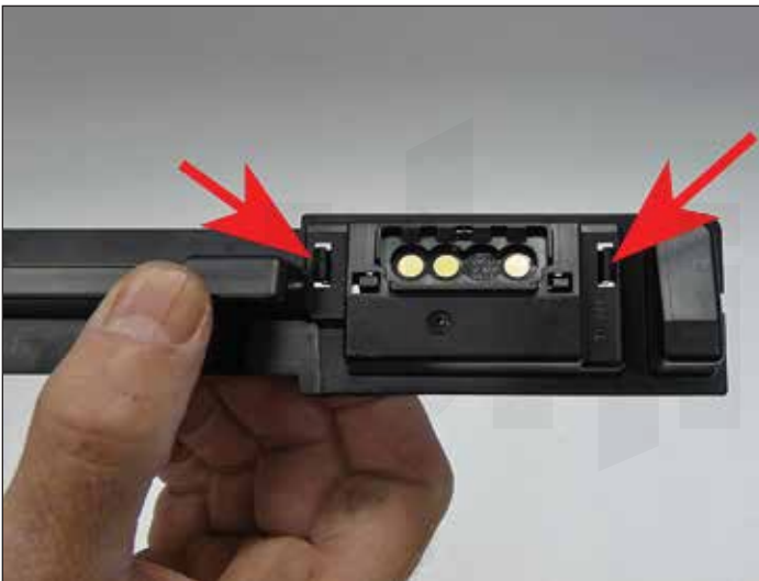
26. Remove the chip holder by pressing in on the two tabs.
