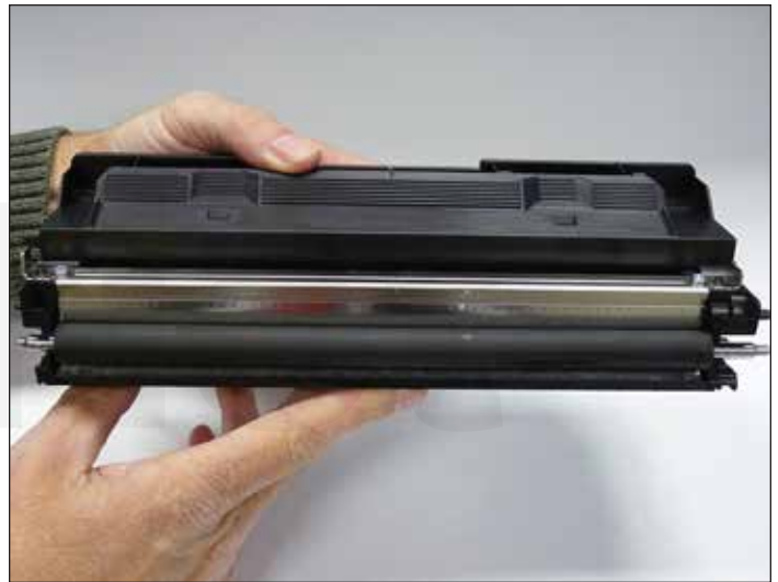
15. Install the cleaned develop roller.
