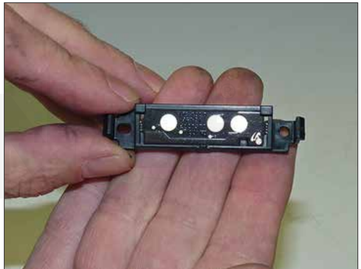
27. On the chip holder, press in on the center tab.
