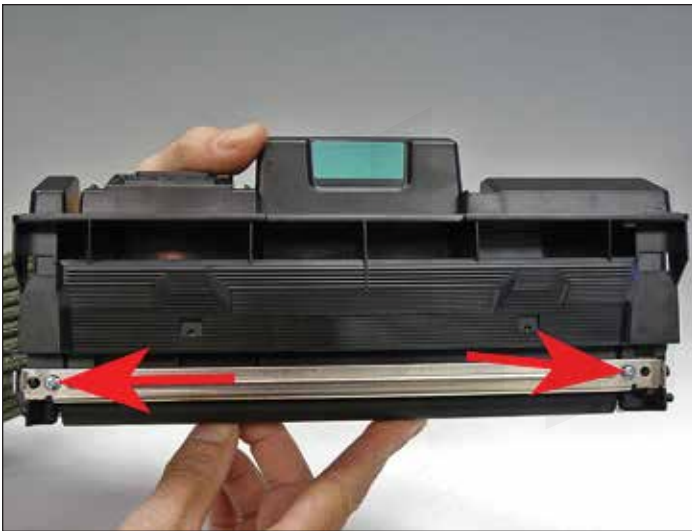
14. Install the doctor blade and two screws.
