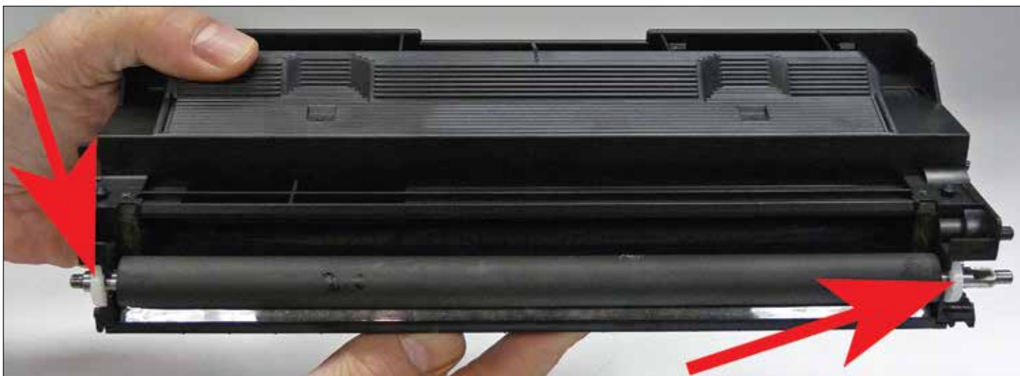
8. Remove the two white plastic washers on both sides of the developer roller.
