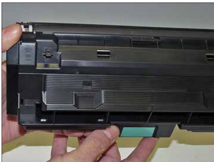
19. Install the top developer roller cover.
