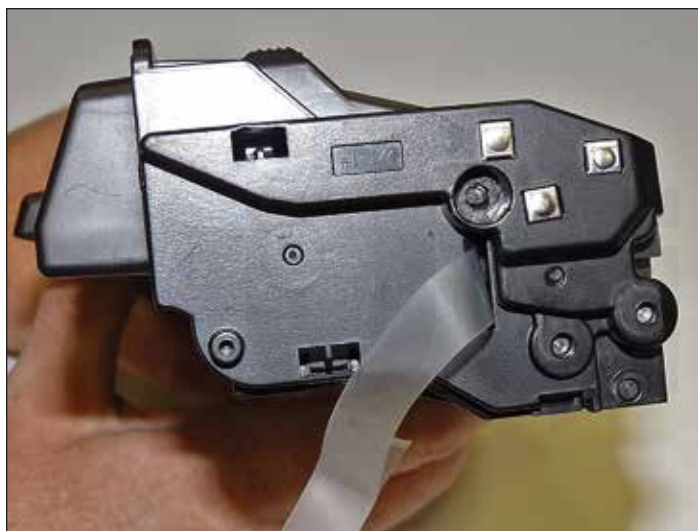
20. Install the contact side cover.
