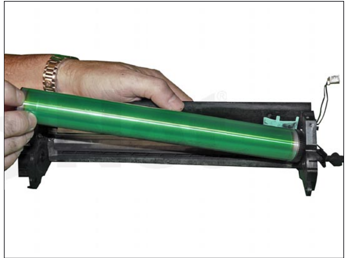
19. Remove the drum.
