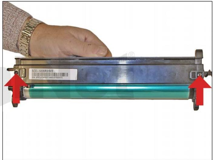
44. Install the PCR assembly and three screws.
