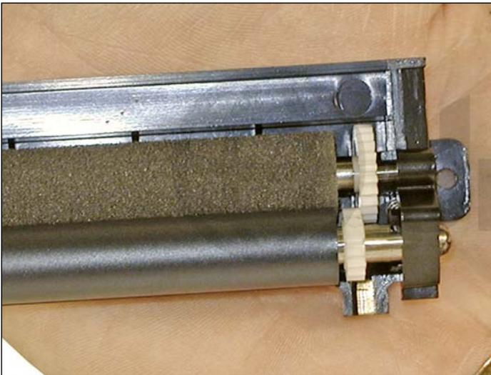
37. On the PCR assembly, gear side, move the PCR drive gear so that it no longer meshes with the cleaning roller drive gear.
