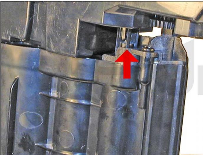
22. Make sure the waste chamber drive gear is meshed with the waste chamber gears.
