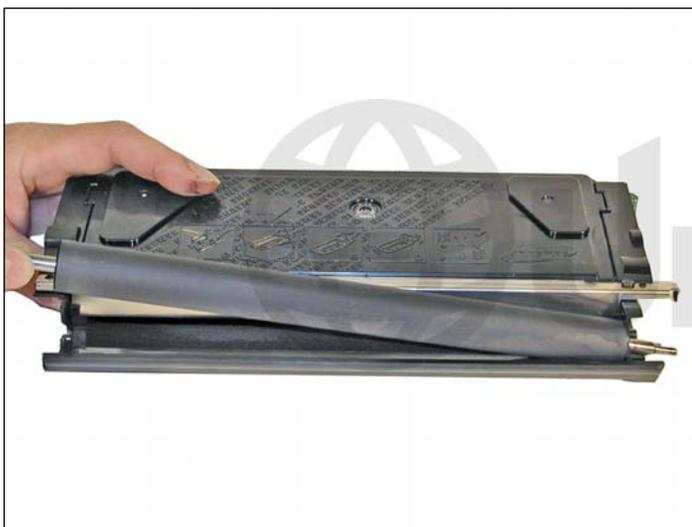
10. Lift the developer roller out of the cartridge.
