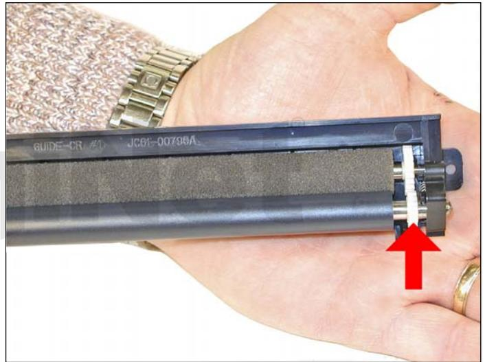
43. Set the two white gears so they mesh again. Failure to do this will allow a buildup on the PCR, ghosting and/or backgrounding will then occur.
