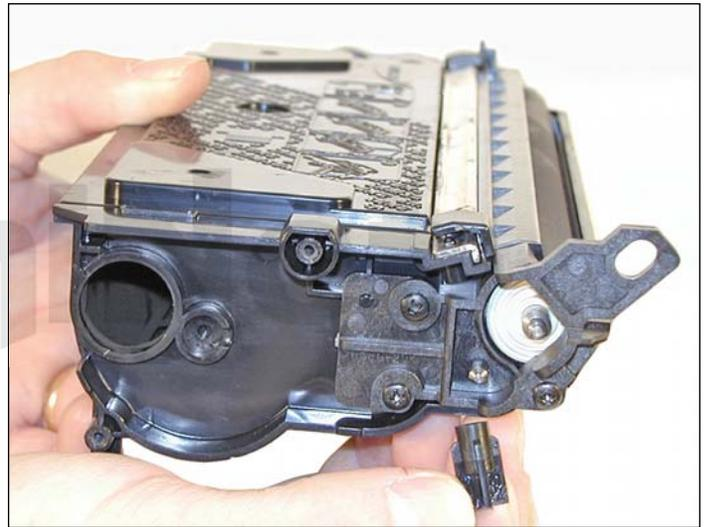
4. Remove the waste chamber drive gear.
