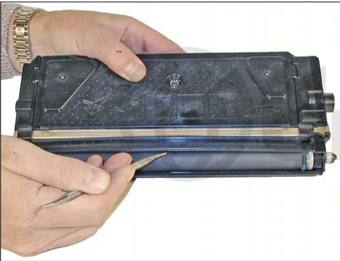
6. With a spring hook, bend up the middle of the developer roller cover, and remove from the cartridge. The cover has a small plastic tab that locks it in place on each side.
