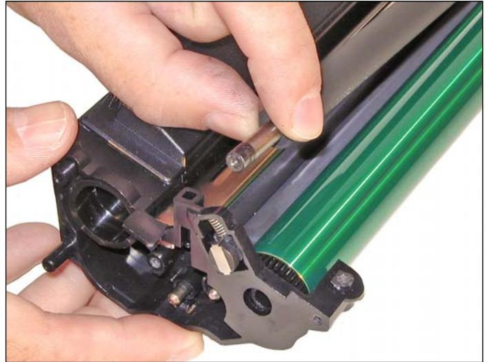
9. Slide the PCR away from the contact side, lift up and remove.
