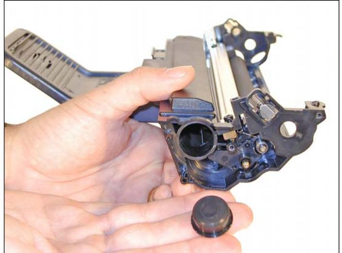
11. Carefully pry out the fill plug. It fits tight and is easily damaged. Work a small jeweler's screwdriver around the edge until the plug comes free.
