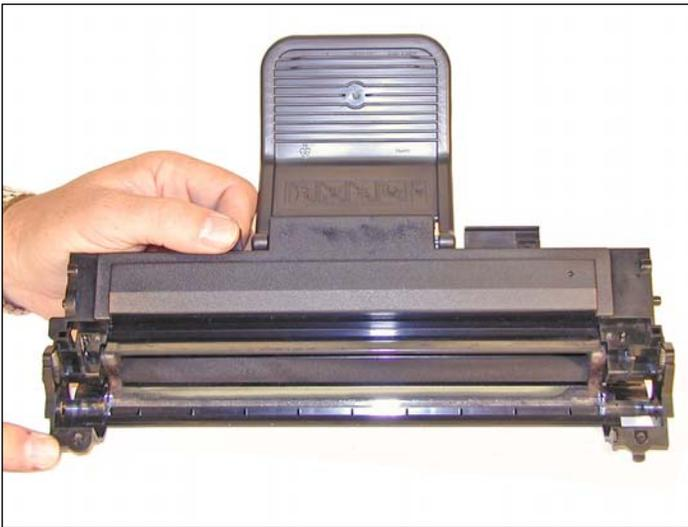
15. Clean the feed roller and any remaining toner from the hopper.
