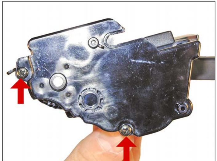
24. Install the gear side end cap, and 2 screws. Make sure the PCR fits correctly in its holder, and all the gears are aligned.
