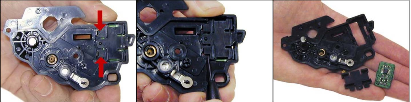
26. On the Non-gear end cap, the chip needs to be replaced before it is installed back on the cartridge. There are 2 tabs that lock the chip housing in. Carefully pry up the two tabs. Remove and replace the chip. Snap the chip housing back in place.
