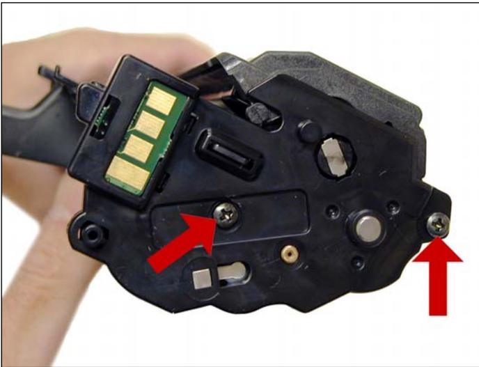
1. Place the cartridge with the handle facing away from you. Remove the 2 screws on the left end cap.
