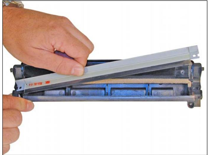
5. Remove the two screws and wiper blade from the waste chamber. Clean out any remaining toner from the waste chamber.
