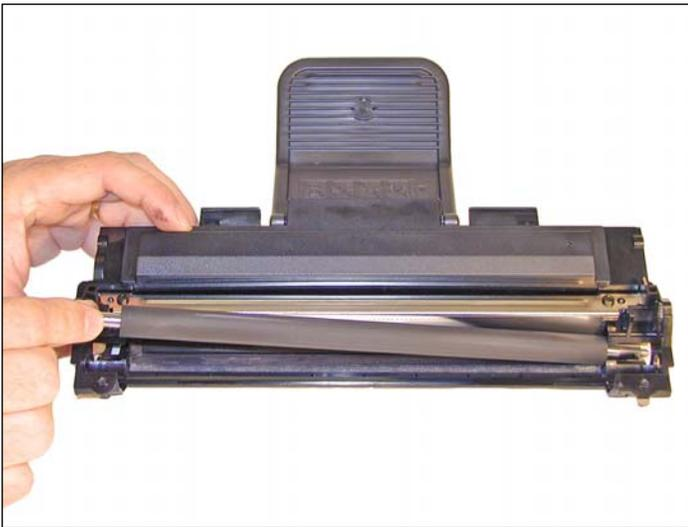
13. Remove the Developer Roller by lifting it out.
