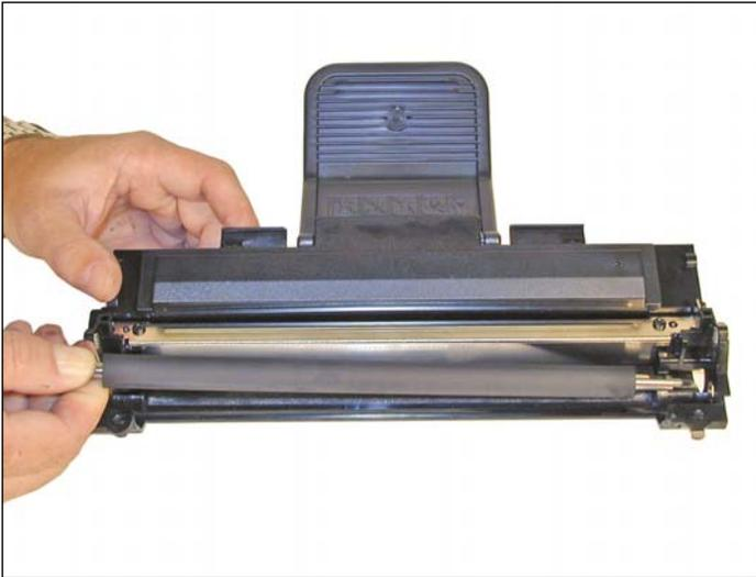
17. Install the developer roller, keyed end to the gear side of the cartridge.
