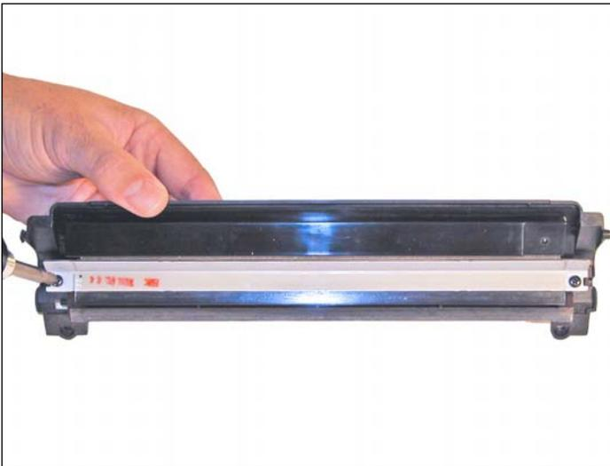
6. Re-install the wiper blade and two screws. Place the waste chamber aside.
