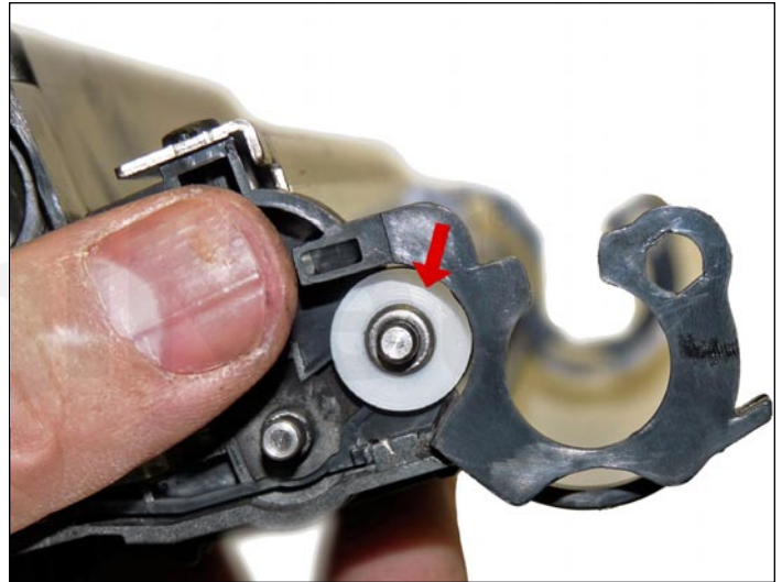
19. Remove the developer roller bushings from both sides.
