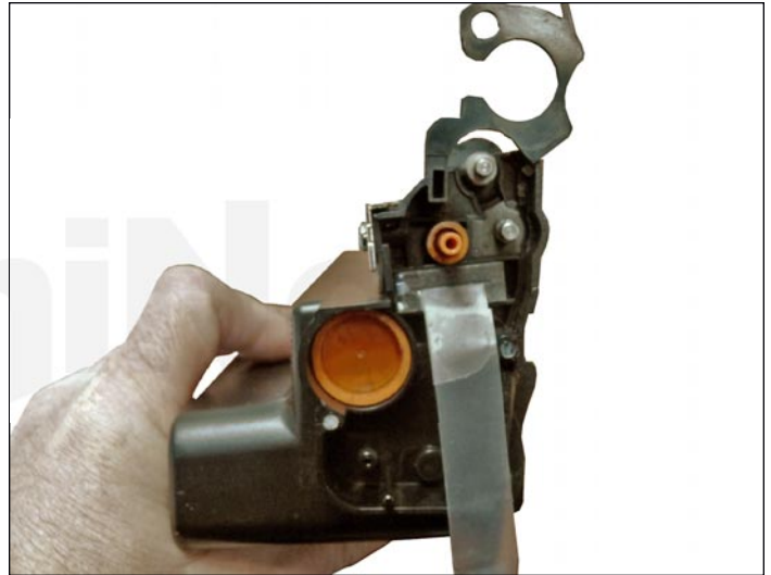
26. Pull the tail of the seal through the seal port.
