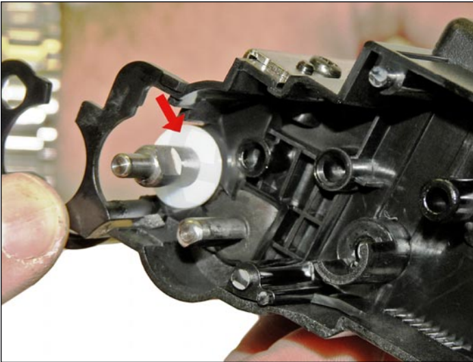
19. Remove the developer roller bushings from both sides.
