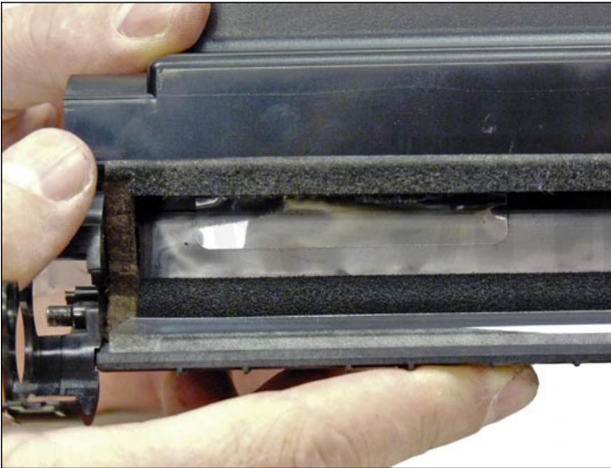
25. Install the seal through the developer roller opening.
