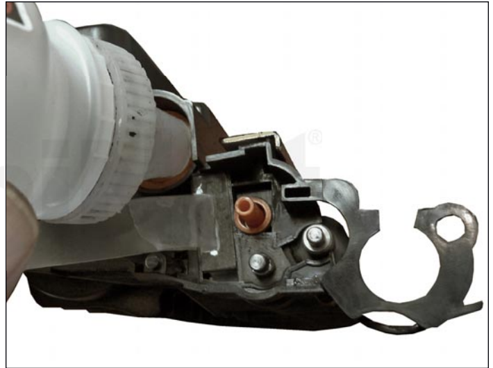
30. Fill the hopper with toner for use in the Samsung ProXpress M3320, replace the fill plug, and check for leaks.
