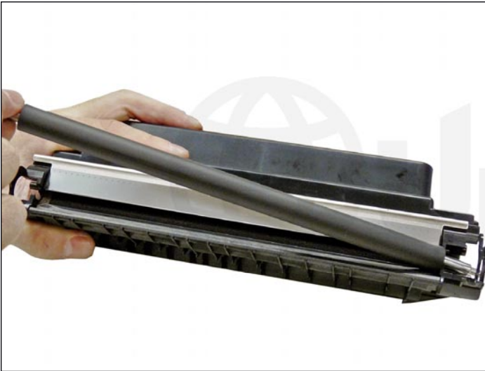
20. Remove the developer roller.
