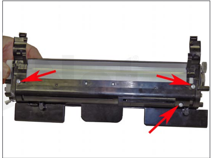
31. Install the bottom cover and three screws.
