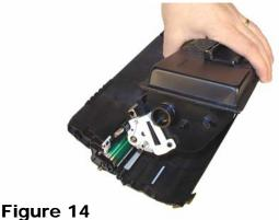
12) On the waste hopper, remove the gold colored screw from the drum axle, work the waste section away from the frame. See Figure 15.
