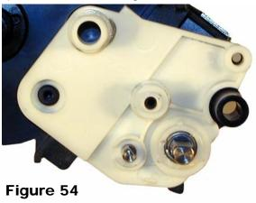
49) Install the center white gear and screw. See Fig. 55
