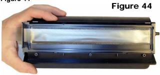
40) Slide the seal tab out the slot of the top cover. Set the three plastic tabs into their slots, and rotate the top cover down into place. Install the screw. Make sure the cover locks into place! Check the seam on the end of the hopper to be sure. See **Figures 45 & 46**
