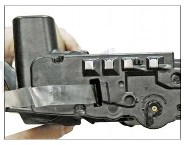
40. Clean the contacts on the left side end cap, and replace the conductive grease.
