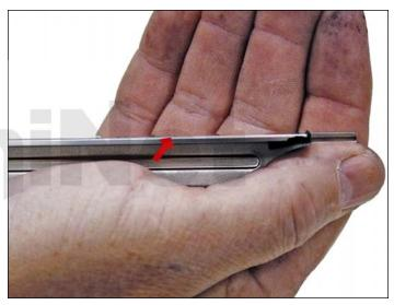
28. Clean the doctor blade edge so there is no evidence of build up along the edge. If any buildup exists, the cartridge will streak. No chemicals should be used. We have found using a clean, wooden ice cream-type stick works great for scraping the blade clean without damaging it.
