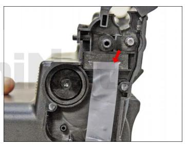
30. Pull the tail of the seal through the seal port.
