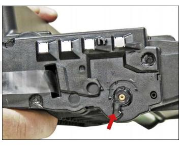
45. The drum separators are fixed to the end caps. They should be set as shown. These arms keep the drum and developer rollers separated until the cartridge is installed in the printer.
