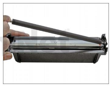
10. Remove the PCR from the assembly. Clean the PCR with your normal PCR cleaner.
