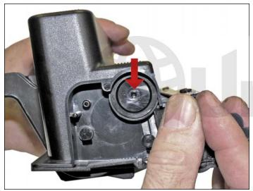
22. On the supply hopper, carefully pry out the fill plug and dump out any remaining toner. The fill plug can be difficult to remove as it is recessed. Take a small common screwdriver and work it around the edge, lifting slightly until it comes loose.
