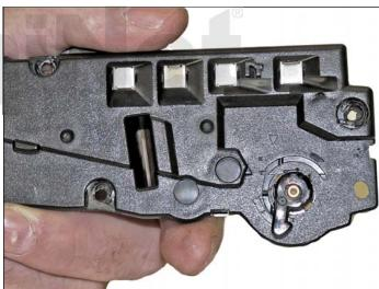
6. On the right side end cap, press in on the three tabs and remove the end cap.
