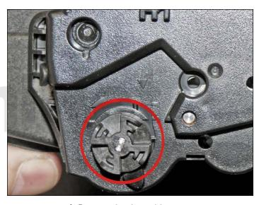
4. Remove the drum drive-gear.
