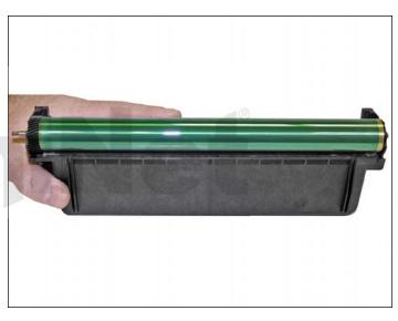
21. Install the drum into the waste hopper, with the large gear of the drum to the gear side (non-chip side).
