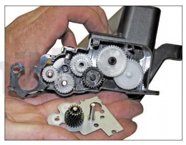
36. Install the gears in the order as shown.
