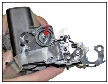
34. Fill the hopper with toner for use in Samsung ML-3712.
