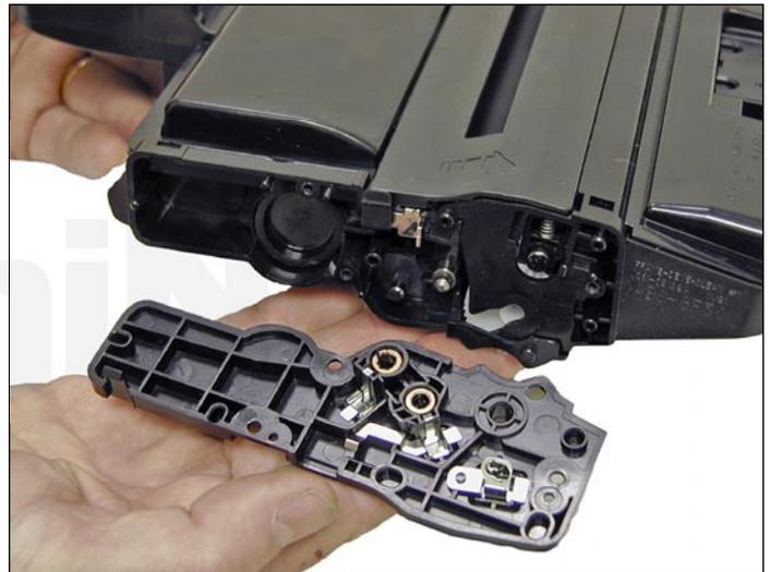
4. On the right side end cap, press in on the top tab and remove the end cap.
