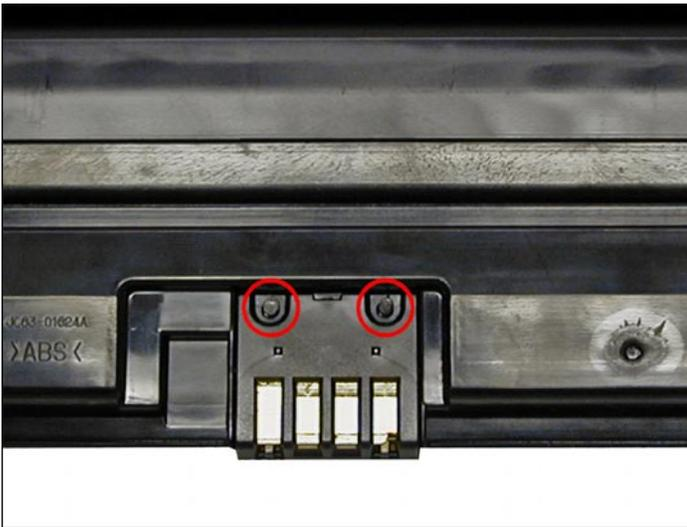
33. To replace the chip, drill out the two plastic rivets with a small drill, remove the cover, and chip.
