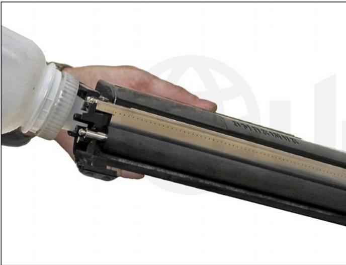
27. Fill the hopper with toner for use in the MLT-D209 toner cartridge, replace the fill plug, and check for leaks.
