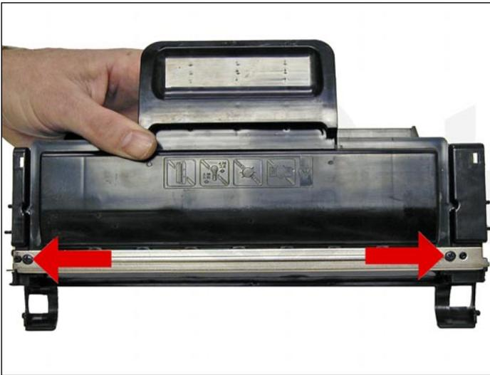
21. Remove the two screws from the doctor blade, and remove the blade.
