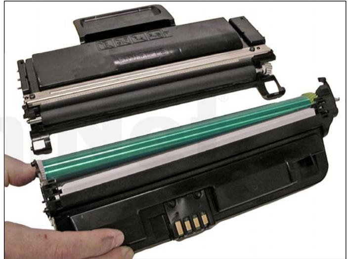
6. Lift up on the drum/waste hopper and remove.
