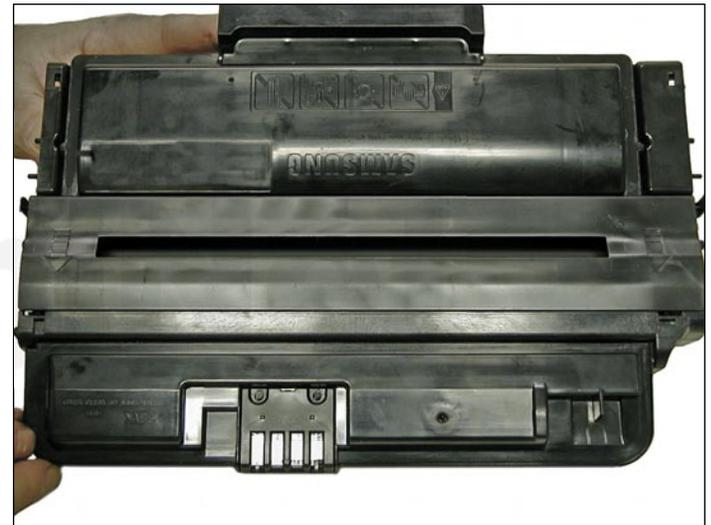
29. Slide the middle top cover/PCR assembly into place.
