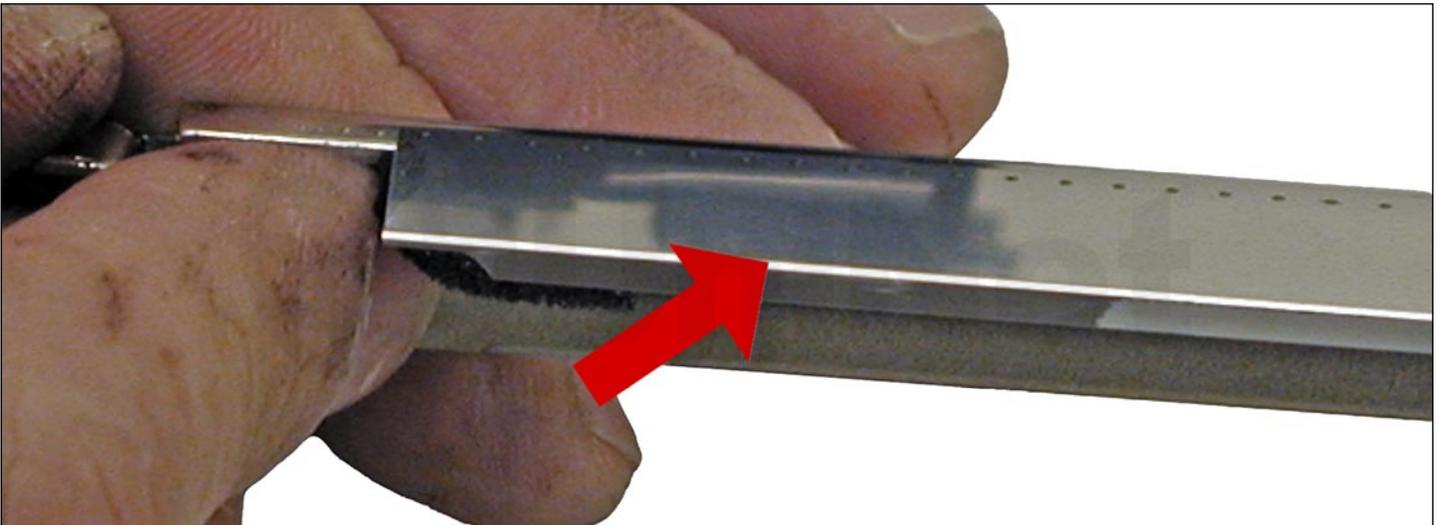
24. Clean the edge of the doctor blade, so there is no evidence of build up along the edge.
