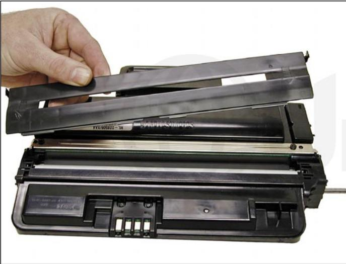
5. Separate the two halves slightly, and lift off the middle top cover.
