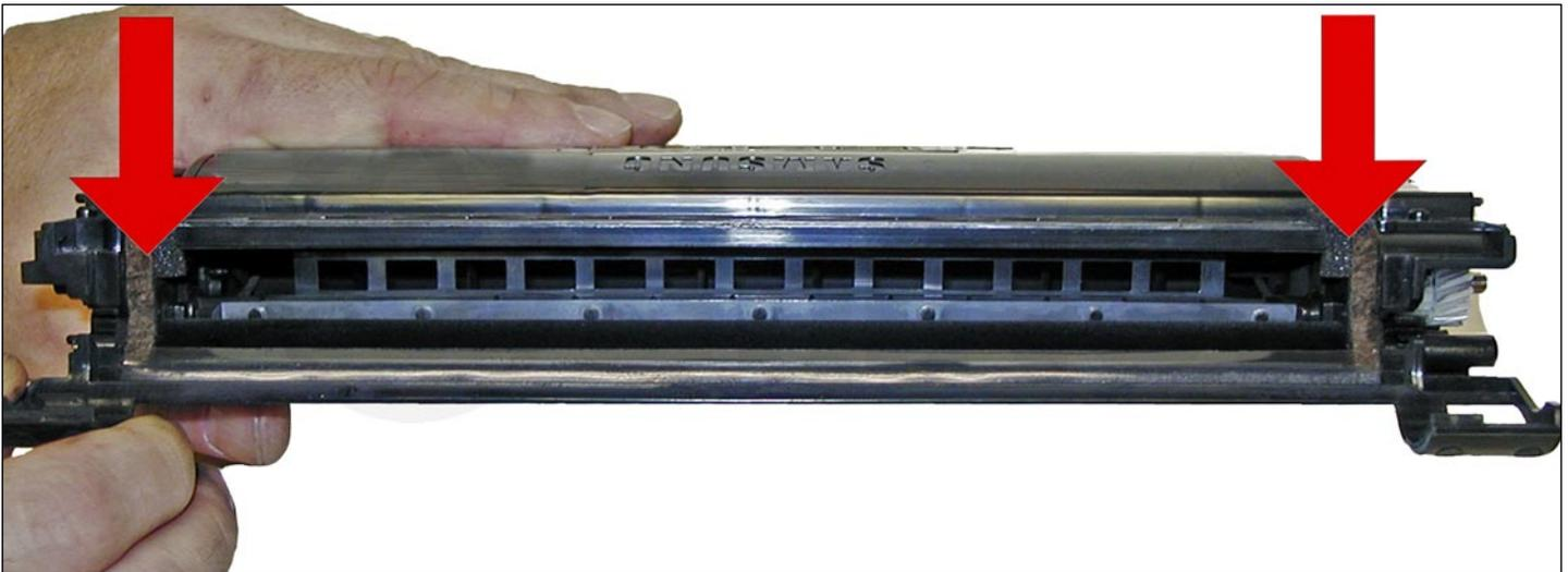
23. Make sure the doctor blade sealing foam and the developer rollers seals are clean and intact.
