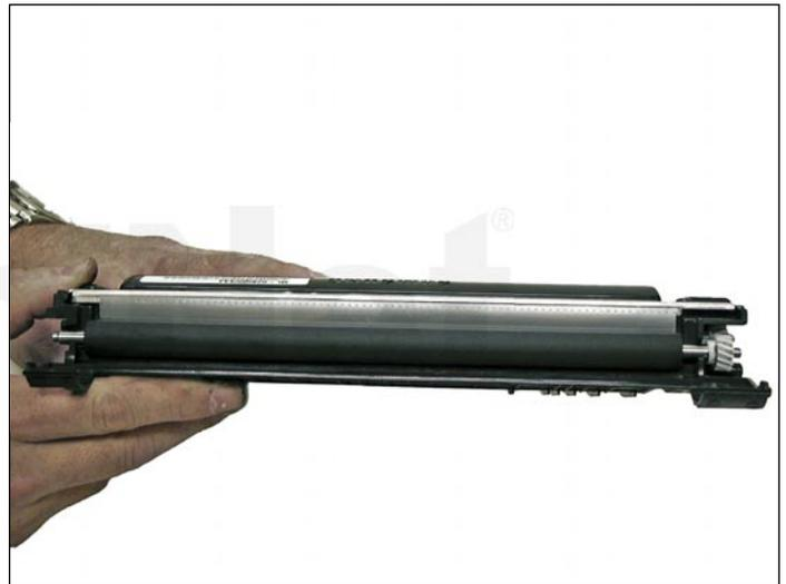
26. Clean the developer roller with a dedicated developer roller cleaner, and replace into the hopper.
