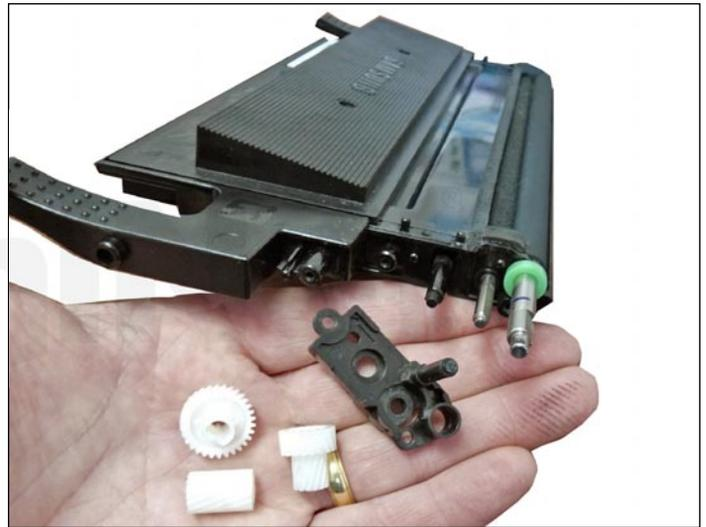
7. Remove the three remaining gears, the two screws and the inner gear plate.
