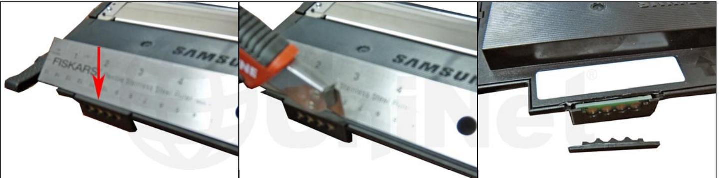
18. To replace the chip, take a small metal straight edge and place it along the cartridge edge as shown. With a sturdy razor knife, cut a line across the chip cover. Remove the straight edge and carefully cut repeatedly along the line until the chip cover has been cut away. Make sure you cut away from yourself in case you slip with the knife!
