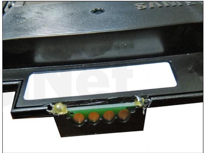
19. Remove the old chip and slide in the replacement chip as shown.
