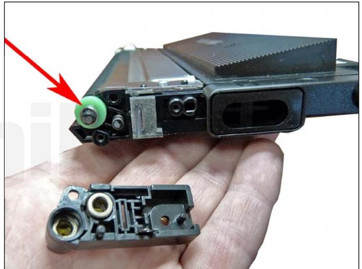
2. Pry off the end cap carefully with a small common screwdriver and remove it. Clean the metal bushings with a cotton swab and alcohol. Remove the green plastic bushing.
