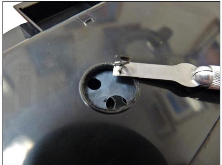
Cheap soldering irons can be modified to use either a copper union as shown or a copper end cap. The soldering iron just needs to have a tip that screws into the end for the end cap, or one that is held in place by a side screw, as we have shown here to use a union. They can be made to melt a cleaner hole by filing the inside edge slightly to taper it in and leave a pointed edge.
