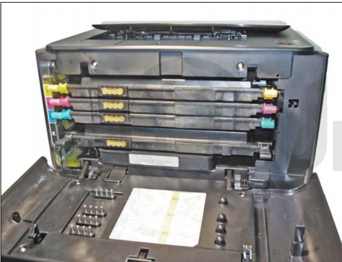
23. Shown are the toner cartridges in the proper order.
