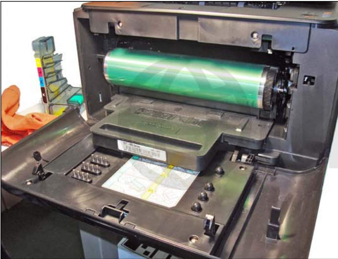
21. Shown is the Image unit installed in the printer.
