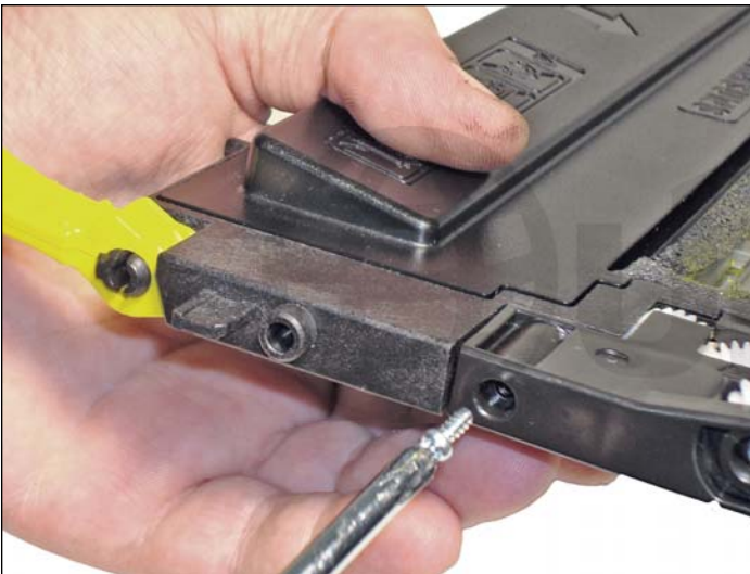
16. Install the opposite side cover with the larger screw as shown.
