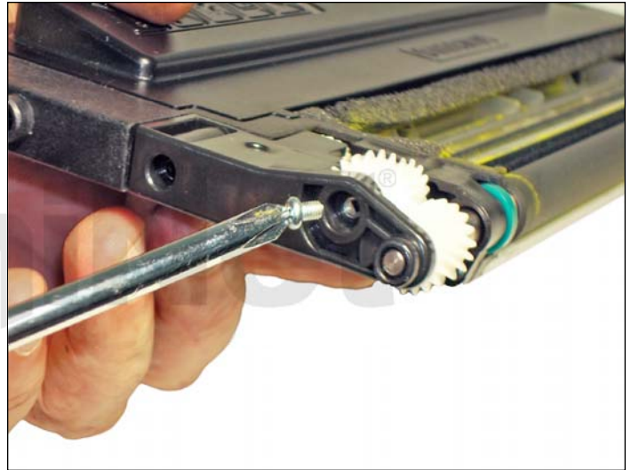
15. Install the cover with the short one with fine threaded screw in the center of the gear as shown.
