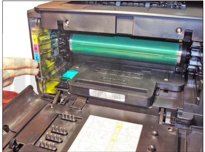
22. Shown is the waste hopper installed (left side). The waste hopper is the left side support for the toner cartridges.
