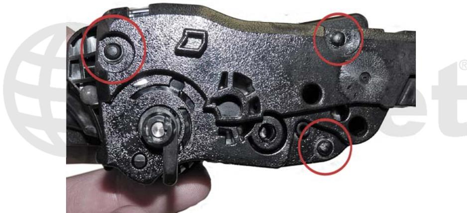
These cartridges, while similar to other Samsung cartridges, have taken a dramatic change in that there are no screws in the outside of the cartridge at all. There are plastic rivets that need to be cut off, holes drilled and screws installed to hold them back on. It's not a hard process and it's covered completely in the instructions.
