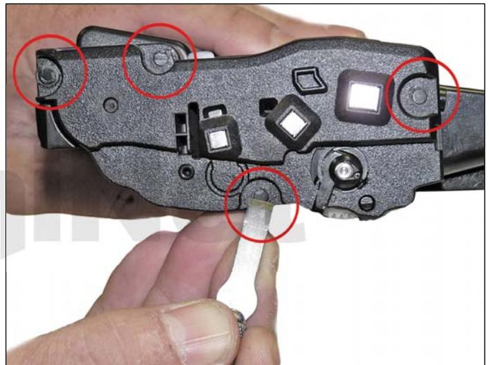
2. On the left side end cap take the chisel blade knife and slice off the heads of the four plastic rivets.
