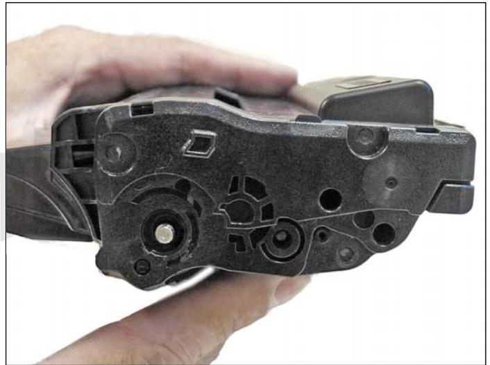
35. Clean the hubs on the gear side end cap, and replace the conductive grease.
