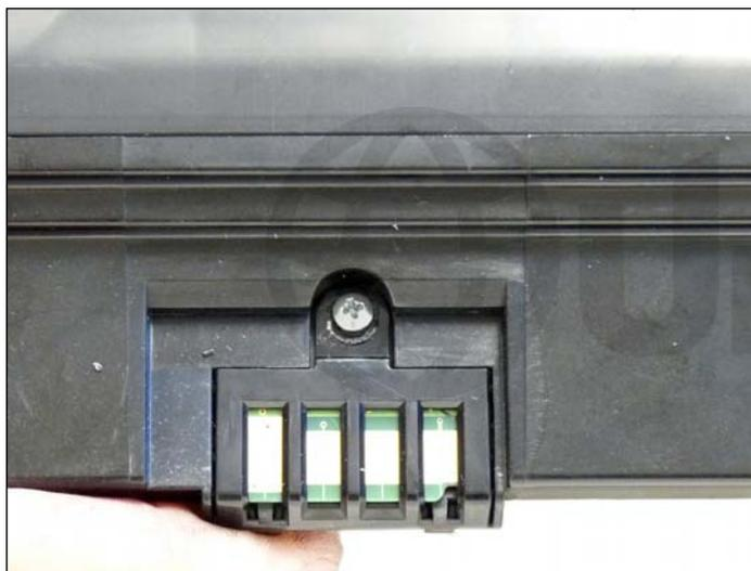
39. Install the new chip and cover. Then, insert a small screw that corresponds to the hole drilled to hold everything in place. It's very easy when drilling the hole for this screw to drill through into the waste chamber. Place a small amount of silicone caulk in the hole and screw before install the screw.
