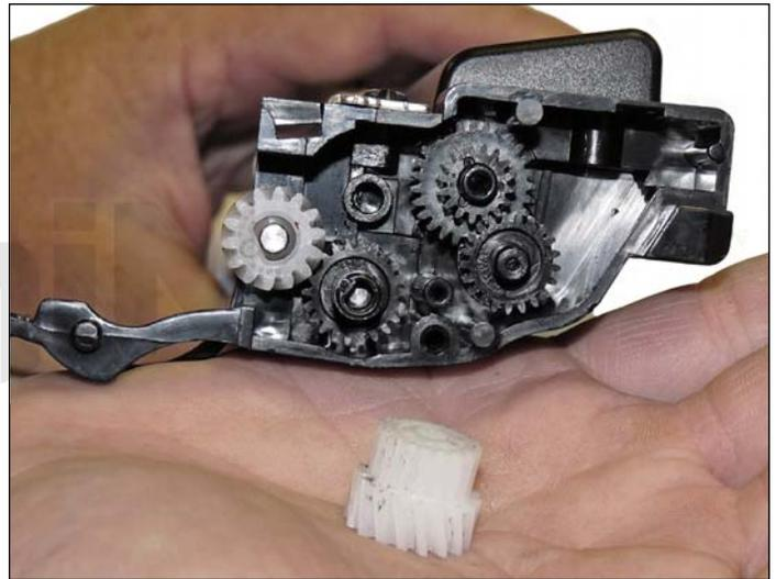
29. Install the gears as shown.
