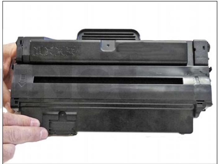
31. Slide the middle top cover/PCR assembly into place.
