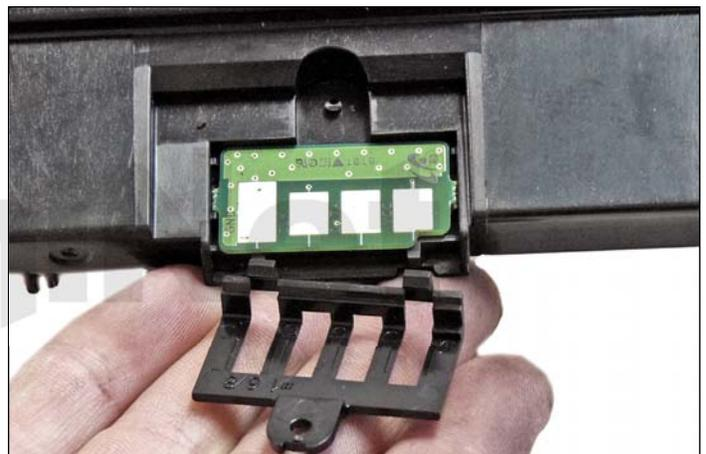
38. To replace the chip, slice the top of the plastic river off with the chisel blade knife.
