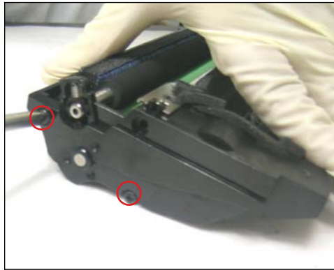
8. Unscrew the two screws as shown to remove the gear-side end cap.
