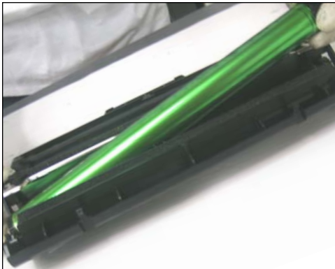
10. Remove the drum as shown. Be careful not to bump or scratch against the doctor blade.
