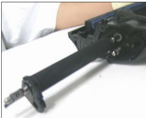
20. Remove the support plate and pull out the developer roller.
