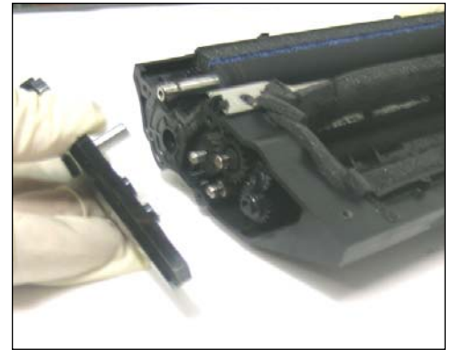
9. Remove the end cap as shown.
