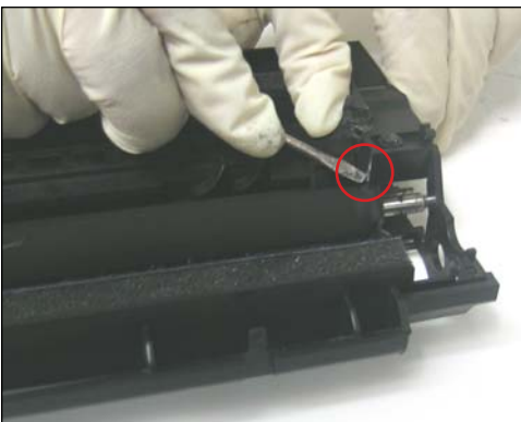
19. Release the second clip located at the opposite end inside just above the developer roller.
