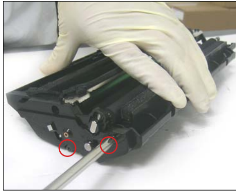
5. Remove the two screws from the gearless side as shown.
