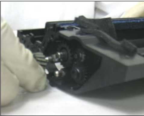
16. Remove all gears as shown.
