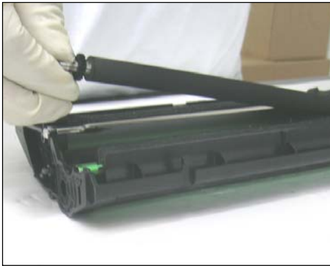
7. Remove the PCR as shown.
