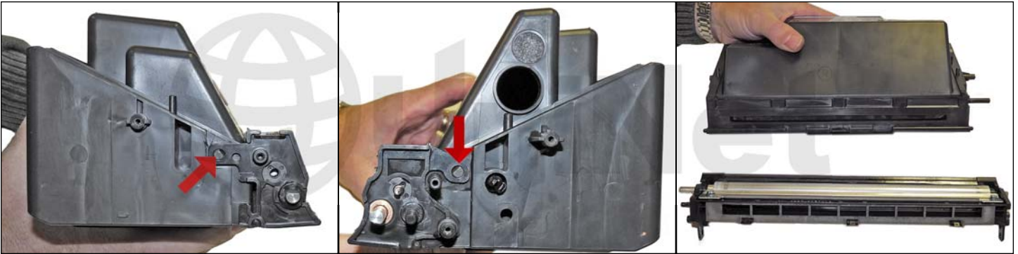
24. Pry up the tabs on both sides of the cartridge to remove the upper magnetic roller section.
