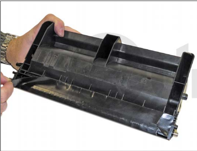
23. Remove the sealing tape from the bottom of the hopper.
