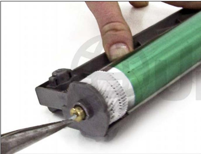
1. Insert a small screw into the drum pin hole shown, turning it clockwise until it anchors in place. Using a pair of needle-nose pliers, grasp the exposed portion of the screw.
