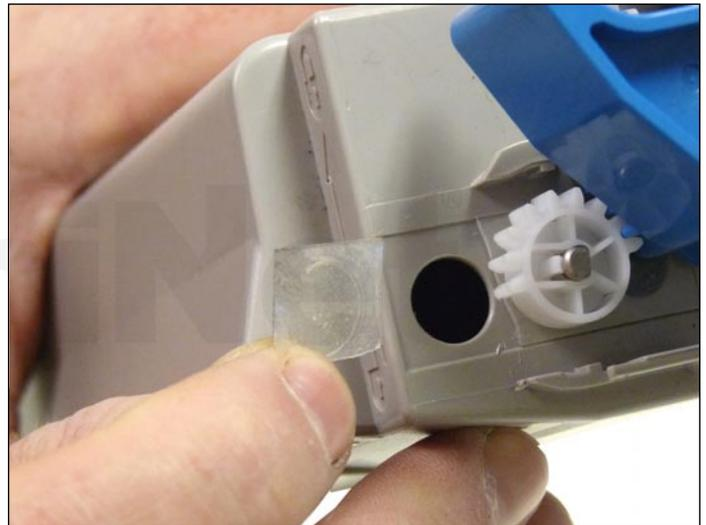
4. Cut the waste hopper seal just past the small white gear.
