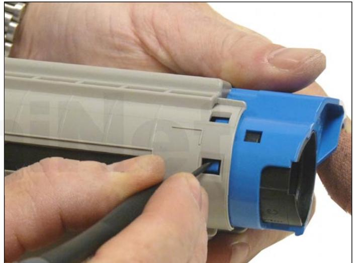
2. Press down on the locking tab of the blue handle. Rotate the handle to open the toner port. Vacuum/blow out any remaining toner.
