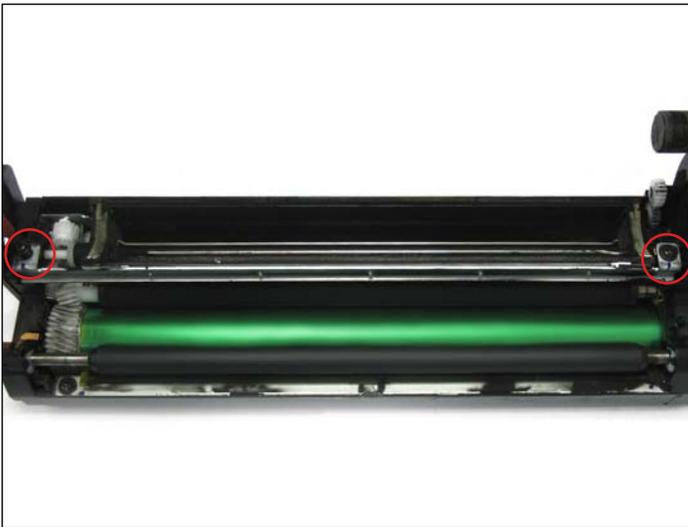
4. Remove the doctor blade by first removing the two screws that hold it in place (as shown).
