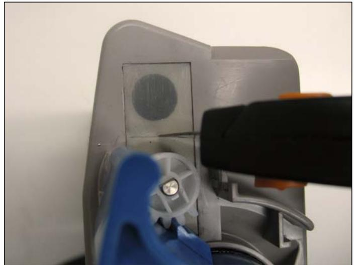
4. Complete removal of the waste section seal cannot be accomplished unless the blue handle is pulled out several millimeters and the small white gear is remove. The next best thing is to cut half the plastic seal in the middle and uncovering one of the holes on the waste section.
