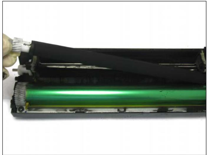
13. Remove the developer roller. Note: Use a lint free cloth to clean off any toner residue. Do not use any chemicals to clean.
