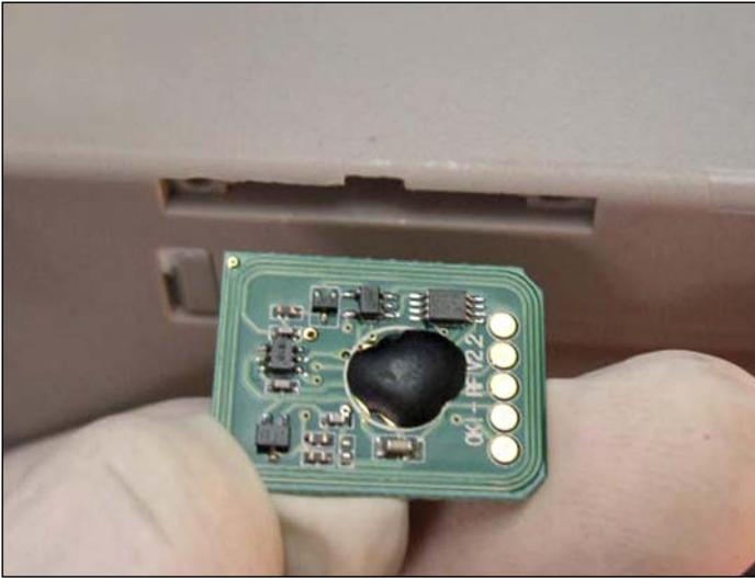
3. Remove the OEM chip from inside the cover and insert the replacement chip.
