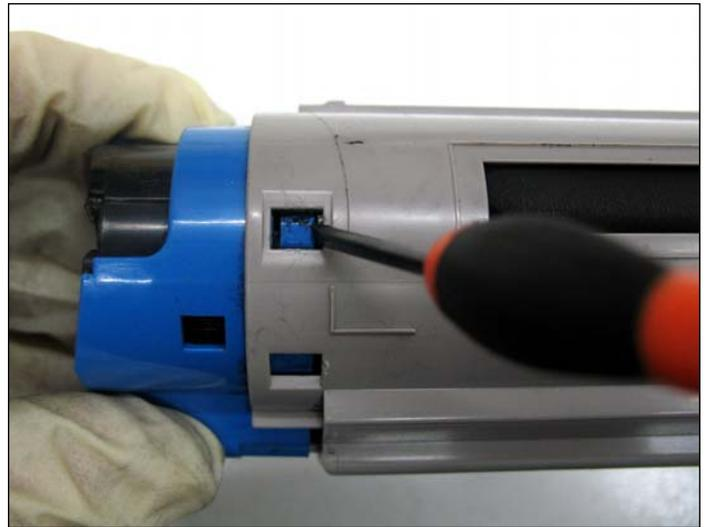
2. Press down on the locking tab to allow the blue handle to rotate to the locked position which opens the feed section. Now you can clean the toner section of the cartridge.
