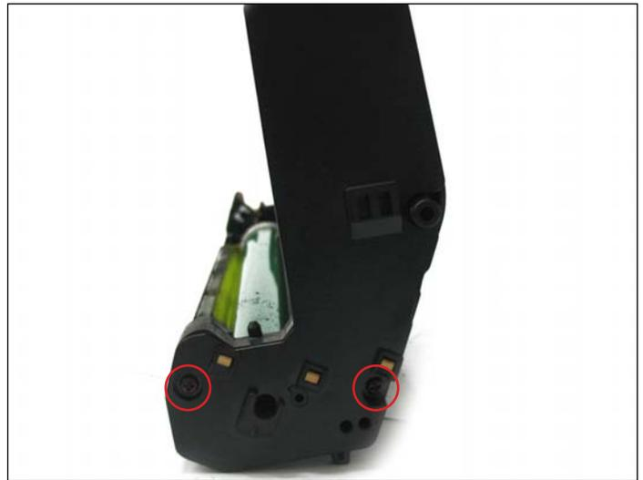
9. Remove the larger end cap by first removing the two screws (as shown).
