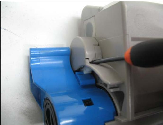
3. Remove the gear cover by using a small flat head screw driver to pry the cover off.
