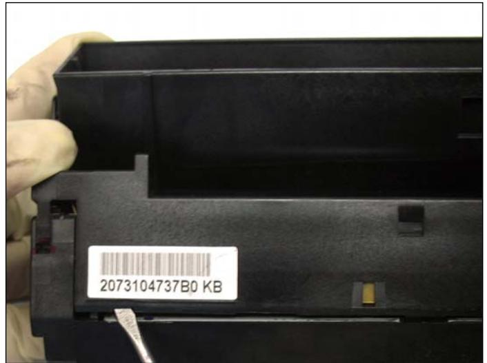
3. Release the front portion of the cover by prying of the left side of the cover first then the right side.
