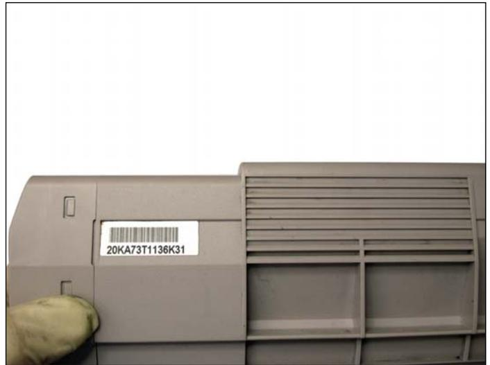
**B. Starter Cartridge Does Not Have a Chip Compartment**
