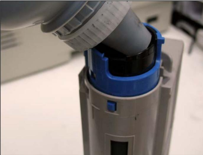
7. Once the cartridge has been thoroughly cleaned reseal the waste opening and turn the blue handle onto the unlocked position to close the feed section. Fill the toner hopper with the adequate amount and install the black plug.
