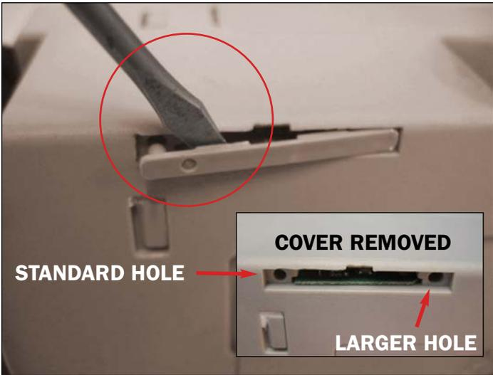
2. Remove the chip cover by inserting a small flat blade screwdriver into the appropriate cartridge opening shown. Slowly pry the cover back to release the clips holding the cover in place.
