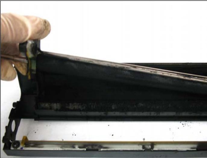
16. Now remove the supply roller assembly and clean cartridge thoroughly.
