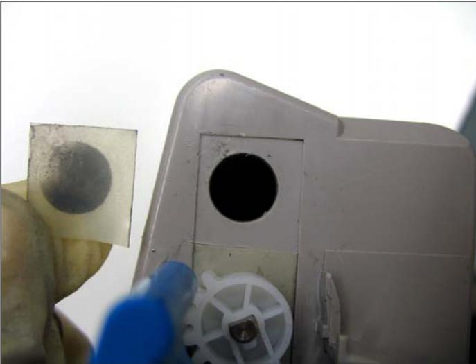
5. Plastic seal removed. NOTE: Empty as much toner possible, before using compressed air to clean the cartridge.
