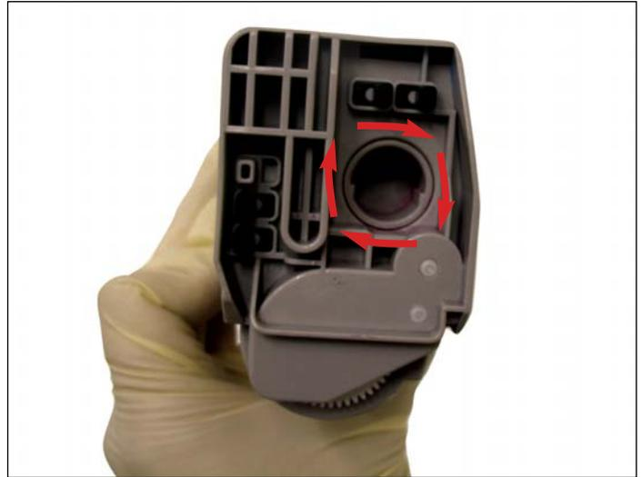
6. With the blue handle in the locked position, the trap door on the waste section (pictured) would rotate clockwise to the open position, allowing you to blow out all the waste toner from the chamber.
