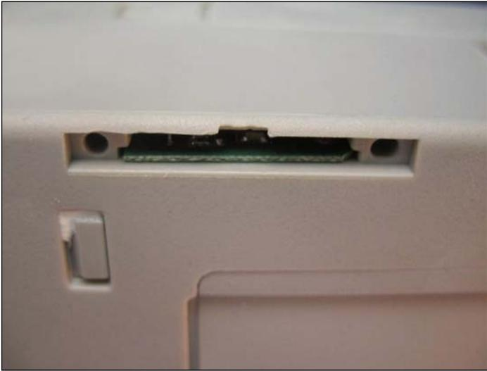
4. Position the new chip correctly and slide into the opening.
