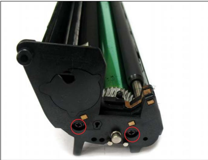
6. Loosen the small end cap to by removing the two screws (as shown) that hold it in place.
