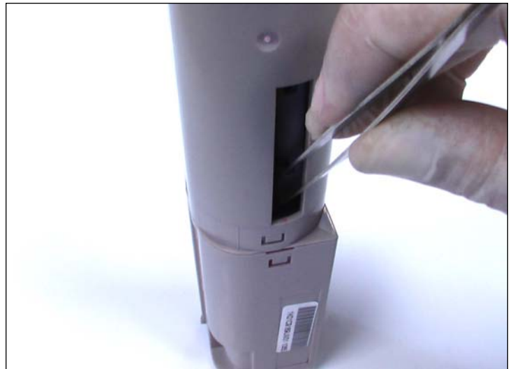
12. Ensure the stabilizer bolt is properly installed by means of pushing it. If it falls during the remanufacturing, reassemble it.
