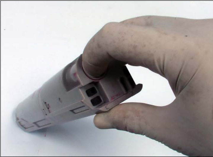
5. Remove the waste hopper section cap by turning it 90° clockwise.
