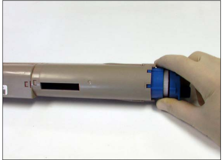
14. Install the blue end-cap and leave the hopper hole free.
