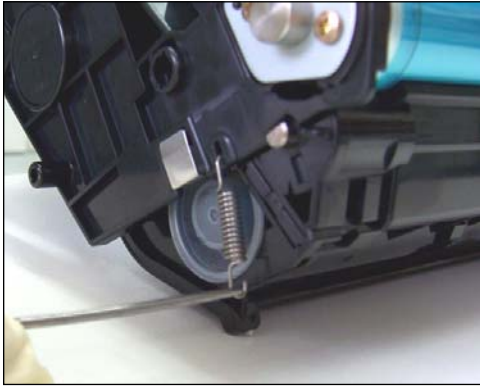
13. Use a hook tool to release the spring from the gear-less side.
