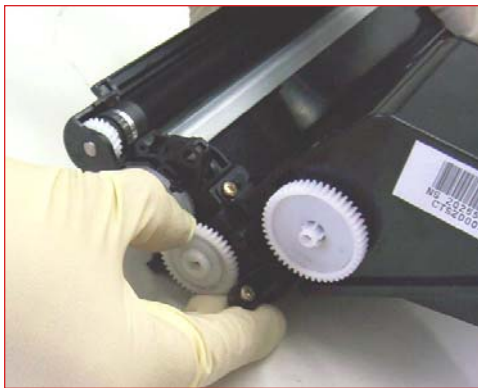
These gears are designed to fit one way, so reinstalling won't become too difficult.
