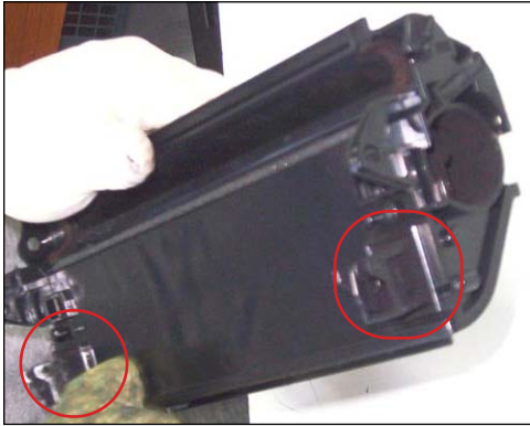
48. Toner hopper removed. Note the two foam seals located at the bottom of the hopper.
