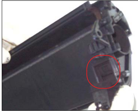
49. These foam seals surround holes where toner passes through to the developer roller. Residual toner can build up in these areas, so it is important to clean thoroughly before reinstalling the hopper.
