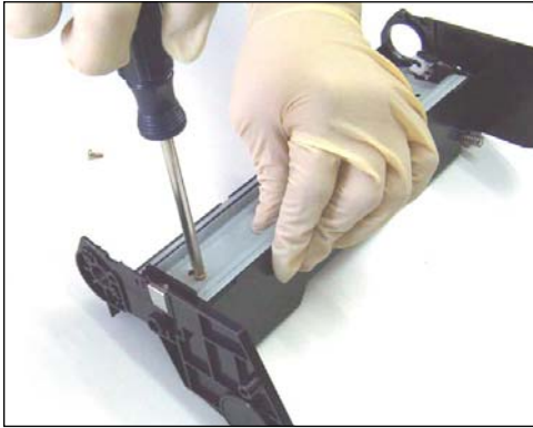
30. Reinstall the wiper blade back into position with the two gold-colored screws as shown.
