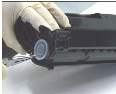
45. Using a pair of needle-nose pliers, remove the two toner fill plugs located on the gear side.
