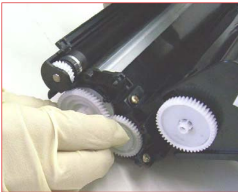
These gears are designed to fit one way, so reinstalling won't become too difficult.
