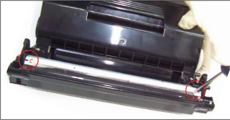
43. Unscrew the two gold-colored screws that hold the the Doctor Blade in place as shown.
