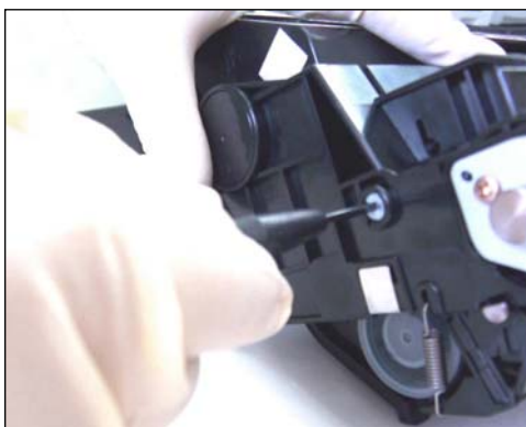
8. Use a 2.4 mm screwdriver to turn the pin to the "release" setting (turn counter-clockwise sensitively until it stops).
