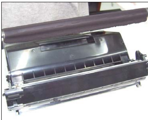
41. Continue with the other side until the MAG is completely removed.
