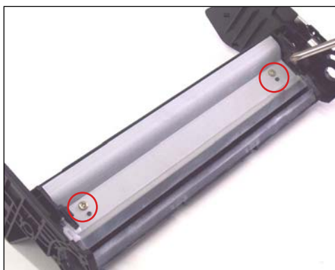
25. Remove the wiper blade by unscrewing the two gold-colored screws at each end that hold it in place as shown.
