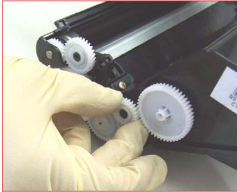
38. Remove all gears from the cartridge as shown in the following photos.
