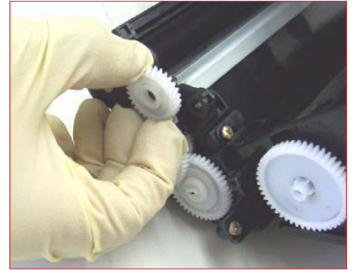
38. Remove all gears from the cartridge as shown in the following photos.
