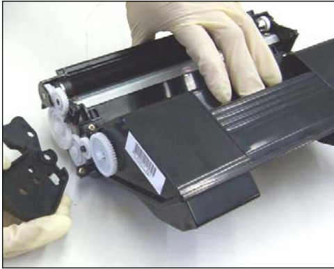
37. The end-cap should then slide out.
