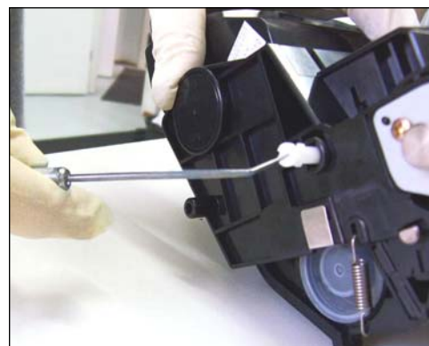
9. Use a 2-angle hook to access and pull the pin from the hole.
