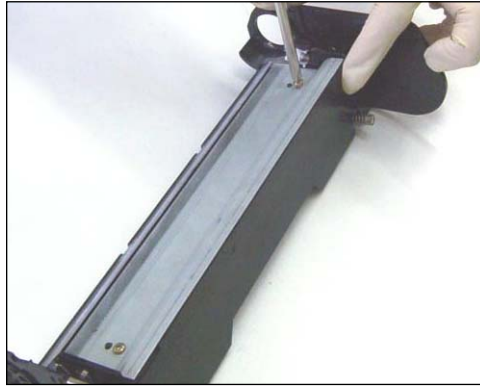
30. Reinstall the wiper blade back into position with the two gold-colored screws as shown.
