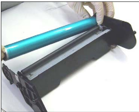
32. Reinsert the OPC gear side first.
