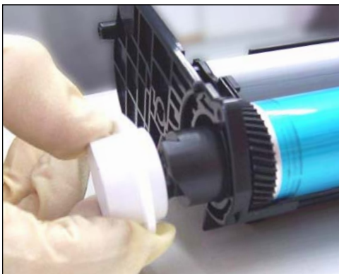
19. Remove the drum gear holder by pulling it out.
