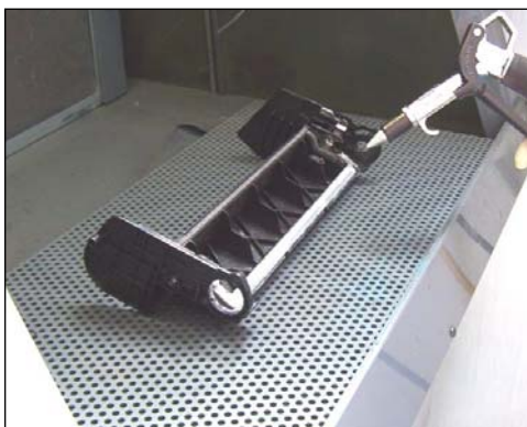
28. Use air pressure to blow out any remaining toner.
