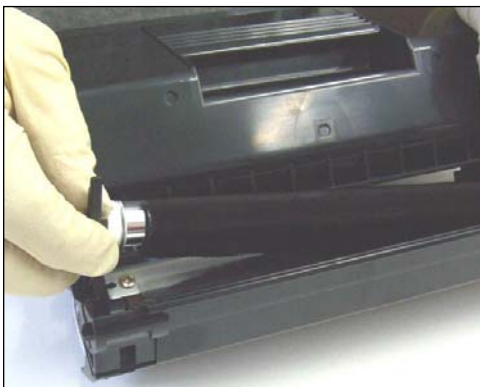
40. When the lever has been flipped up, lift that side of the roller first.
