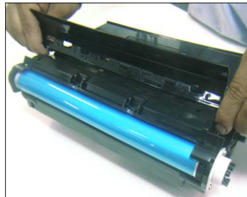
6. Remove the shutter-door and set it aside.
