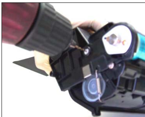
7. Remove the plastic pin on one end by first drilling a hole in the center of it. This will make it more accessible.
