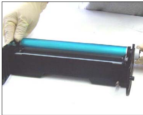
33. Reinstall the remaining drum holder on the opposite side.
