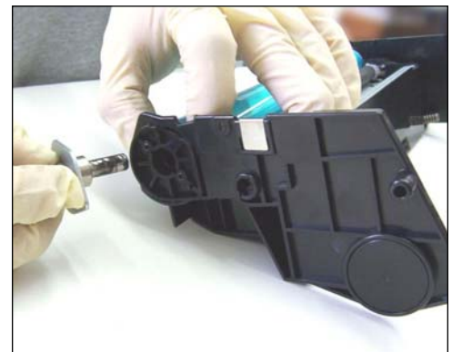
21. Remove the drum pin by pulling it out.
