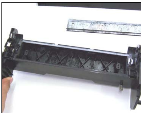
27. You are now ready to clean the wiper blade and waste hopper.
