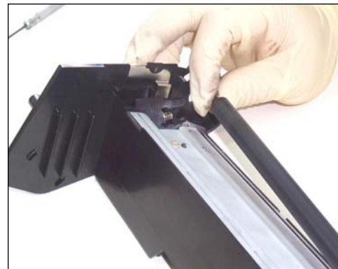
24. Remove the PCR by un-clipping it from the white and black holders.
