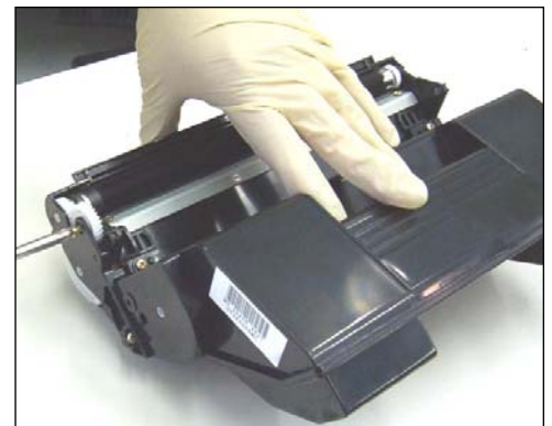
36. Remove the end-cap on the gear-side of the toner cartridge by first removing two gold-colored screws as shown.
