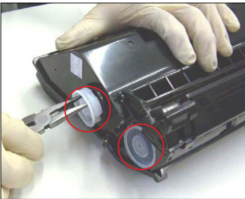
45. Using a pair of needle-nose pliers, remove the two toner fill plugs located on the gear side.
