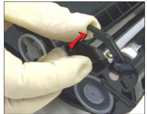
39. Unlock the MAG roller by lifting the lever up as shown.
