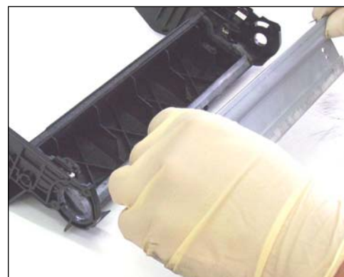
26. Lift the wiper blade evenly from the waste hopper.
