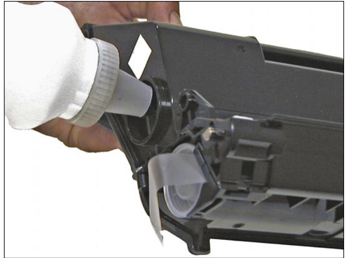
31. Fill with 700g toner for use in the Okidata B700 series toner cartridge in the upper chamber.
