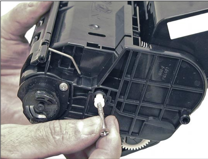
34. Install the two white plastic locking pins.
