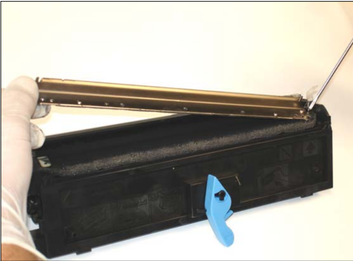
7. Release the doctor blade by lifting it from the left as is showed in the picture. Be careful with the sealing foam under the blade.
