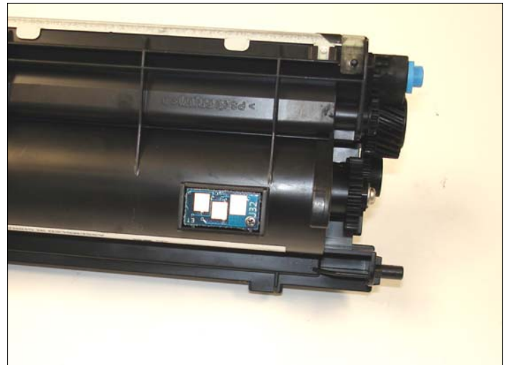
16. Install the Uninet chip and place again the little screw. Finally, install the develop roller cover for shipping.
