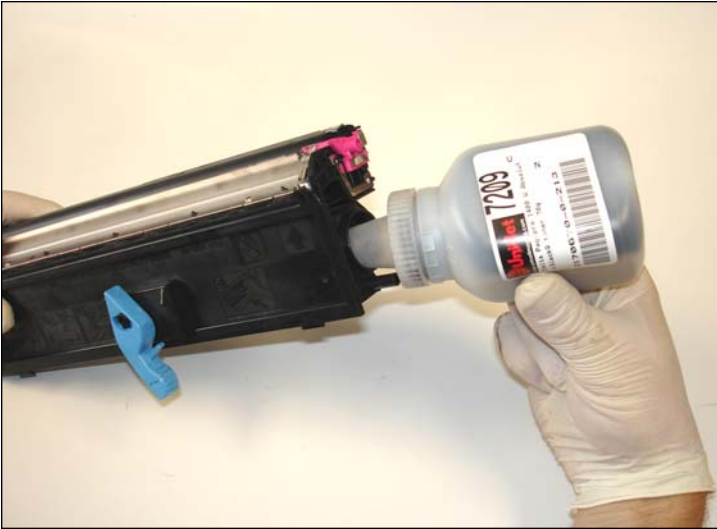
13. Refill the hopper section with toner through the hole. Use a 12mm beak in the bottle and load the proper toner volume.
