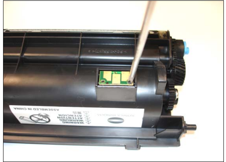
14. Use a screw driver to remove the small screw that secures the chip.
