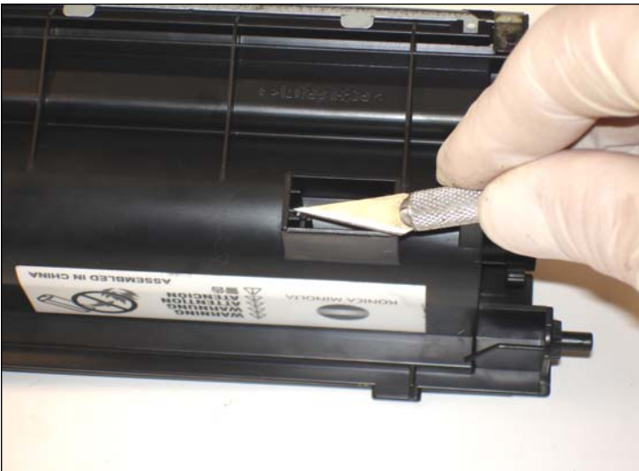
15. Using an X-Acto knife, carefully cut away the melted plastic tab.
