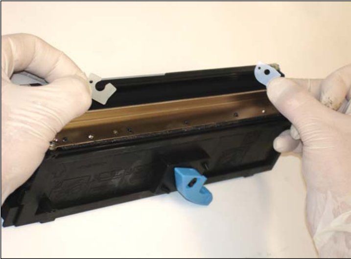
5. Detail of the sealing mylars position. When installing again it must be placed this way.
