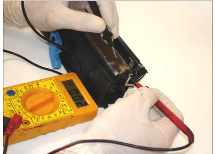
12. Check the electrical continuity with a tester to ensure good contact between the doctor blade and the main contact.
