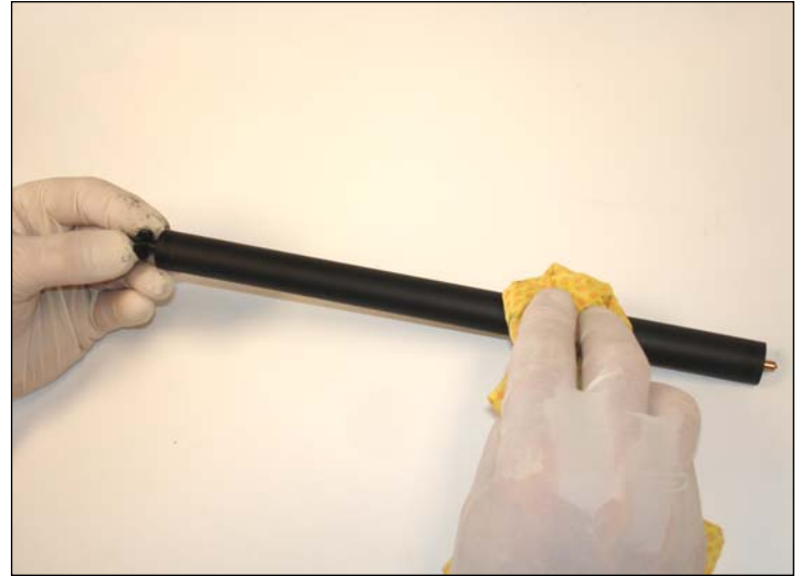
10. Clean the develop roller with compressed air. Afterwards use a lint-free cotton pad with distillate water (70%) and isopropyl alcohol (30%).
