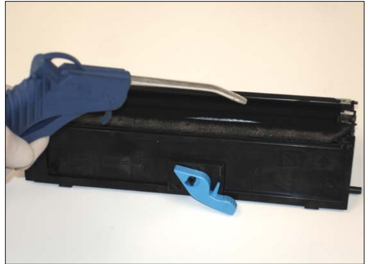
8. Use compressed air to clean residual toner from the toner hopper section. Place the foam properly as a bad installation would cause leaking.
