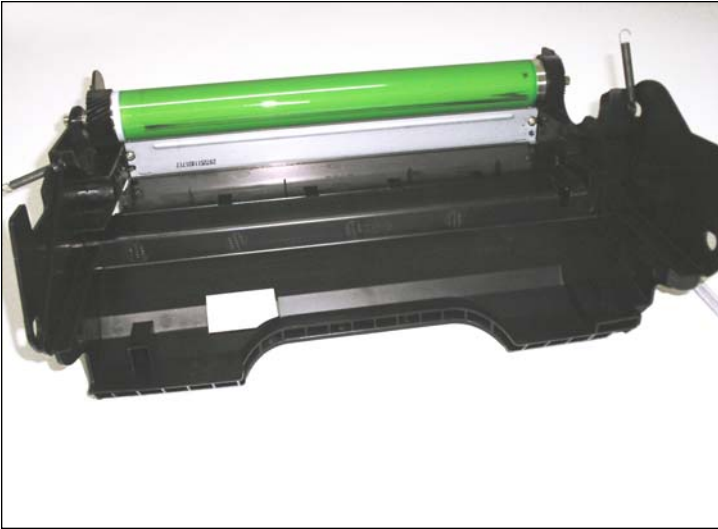
5. Drum unit with hopper section removed.
