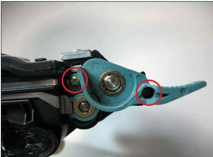
10. Remove the small DVR support plate on the contact side by removing the two screws holding it in place (marked with circles).
