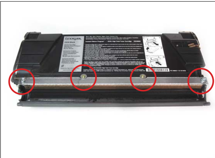
13. Remove the doctor blade by removing the four screws as shown. Note: the location of the doctor bar. It needs to be positioned in the same manner as before.
