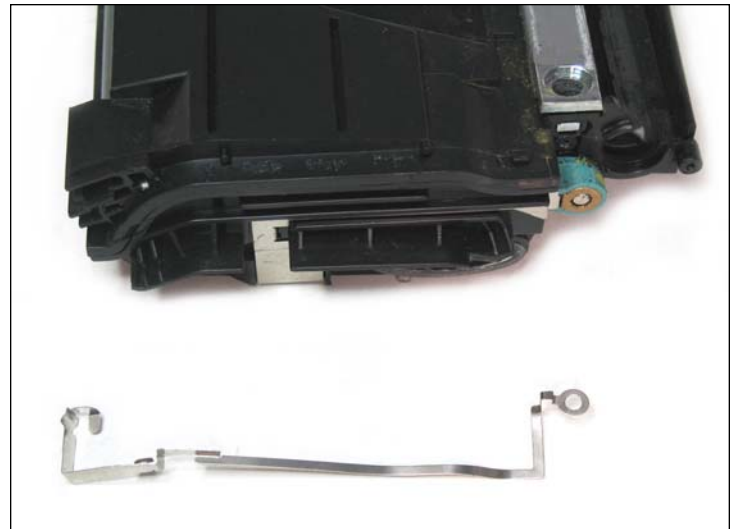
14. Remove the doctor blade contact which runs along the side of the cartridge.
