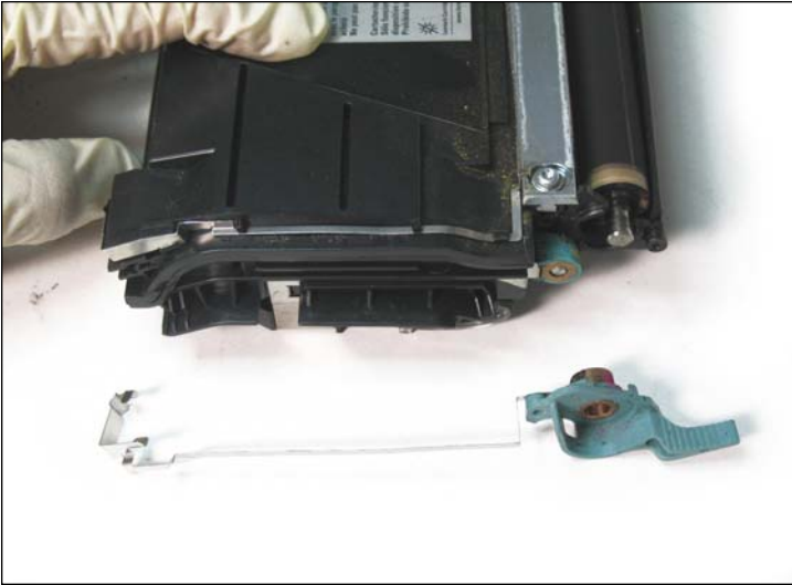
11. Once the DVR support plate has been released, removed with the rear contact as shown.
