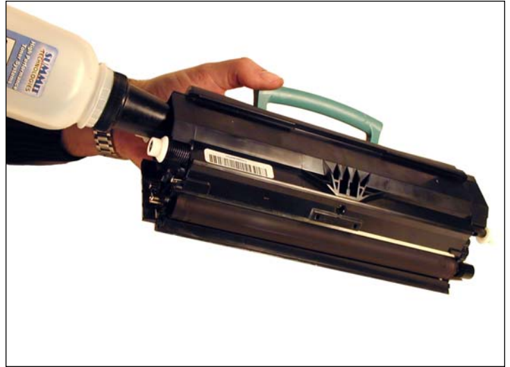
14. Fill the cartridge with the proper amount of toner and install fill plug.
