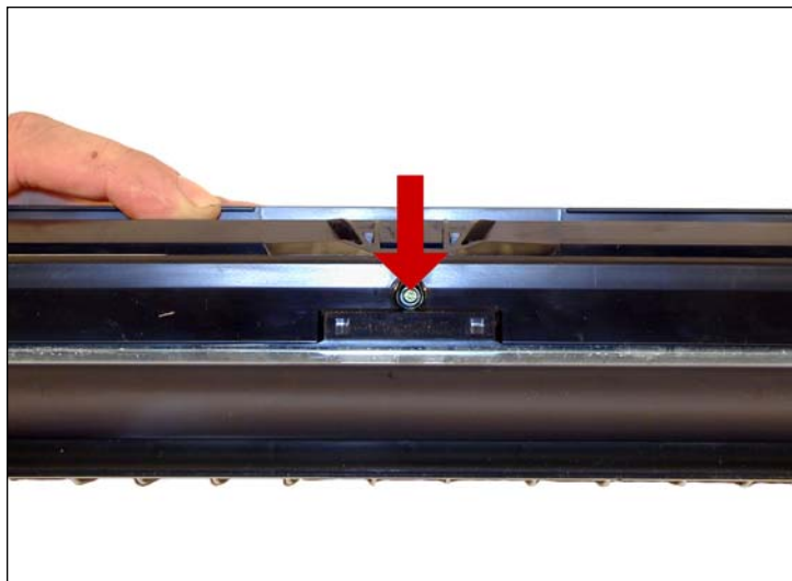
1. Remove the developer roller screw & cover.
