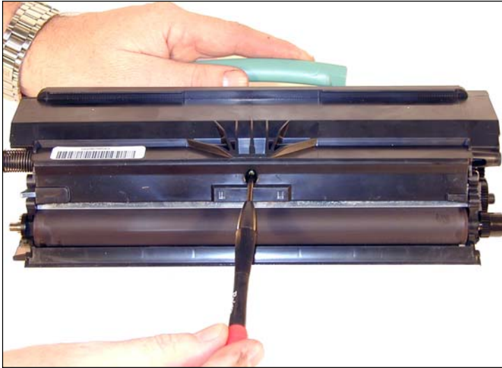
13. Re-install the developer roller cover and screw.
