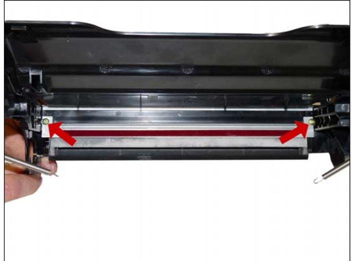
7. On the wiper blade, remove the contact spring. Remove the two screws on either end of the wiper blade.
