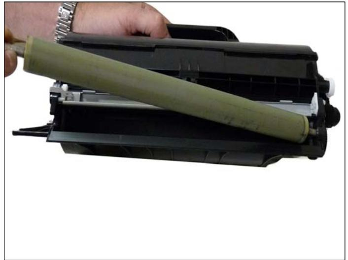
19. Remove the developer roller. Note that there are no spacers on these cartridges. NOTE: Always remove the doctor blade before removing the developer roller. Failure to do this will cause the doctor blade to slide down from its original position and possibly ruin the alignment. Vacuum/blow the toner hopper clean.
