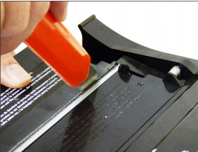
8. Place the cartridge so that the waste bin is face-up. Take a razor blade and cut the foam seal that runs along the back edge of the wiper blade to separate it from the cartridge. Make sure to cut along the plastic/foam and not the blade.
