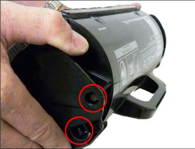
34. On the right side of the cartridge, pull the cartridge shell out so that the right side post falls into its slot.
