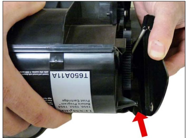
2. There are two plastic posts from the hopper that fit into the cartridge shell. Pull the edge of the shell out to release the posts, and lift up the hopper so that the posts are free.
