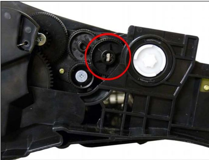
36. Re-install the developer roller drive gear. Hold the gear train and turn the gear until it locks. It's a little hard to get on now than if installed before, but it's easier to install the hopper this way. Either way is fine though.
