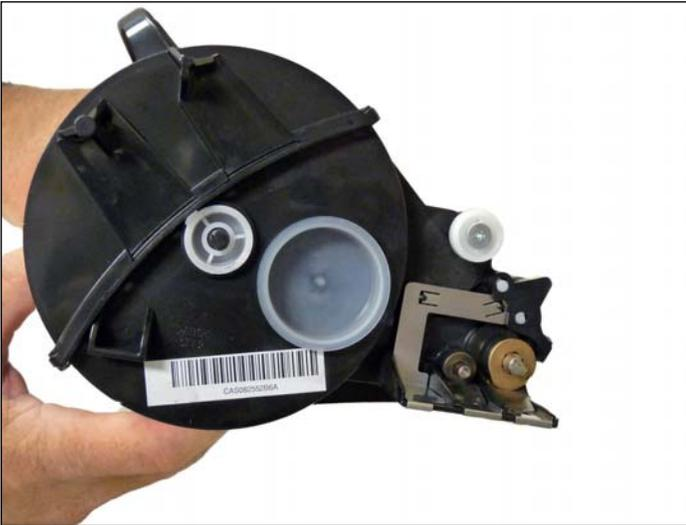
14. Remove the fill plug from the hopper.
