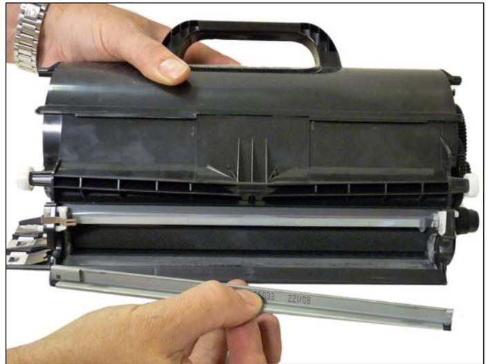
21. Remove the doctor blade by sliding the blade down out of the track.
