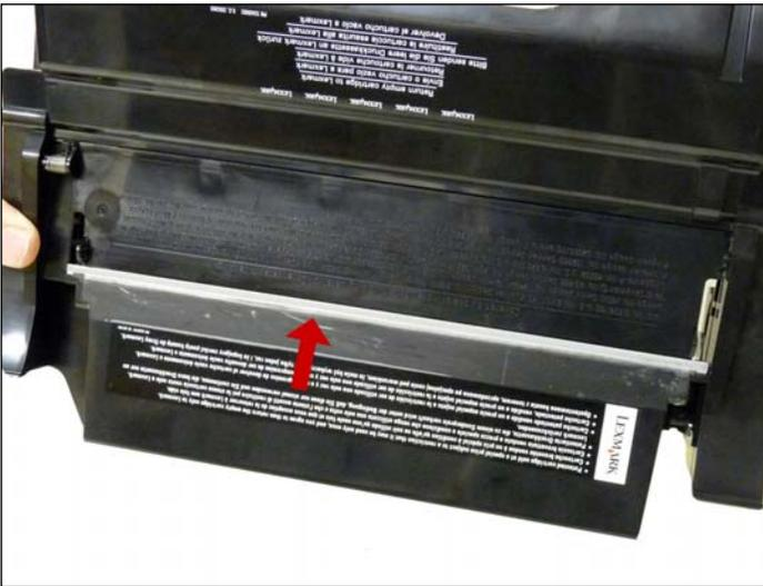
12. Place a piece of clear tape along the edge of the wiper blade. If the tape does not stick well, the area should be cleaned with alcohol. It is very important to get a good seal with the tape, otherwise the cartridge will leak. Trim away any excess tape. Be careful not to allow any tape into the laser port opening.
