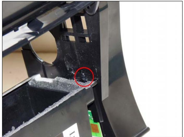
9. Hold the cartridge so that it is upright (standing up with the waste bin on the table). With one hand, hold the laser shutter open, and with the other hand, remove the wiper blade. Work the blade off carefully so that the alignment pin does not break!
