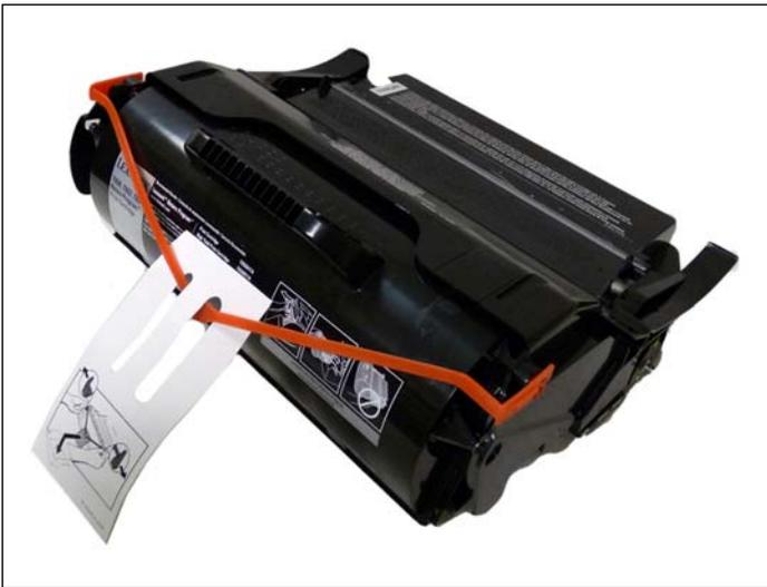
38. A shipping lock must now be installed. This lock should be used even if you are going to hand deliver the cartridge. It will prevent the toner hopper from coming in contact with the OPC drum, and causing damage to either the drum or the developer roller. Press the two red tabs into the sides of the cartridge as indicated in the picture supplied with the lock.
