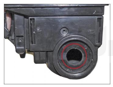
1. Drill a 1/2" to 3/4" hole into the fill plug.
