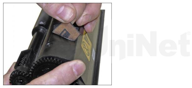
5. Peel off the old chip label (it is an RF type chip).
