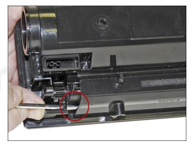
2. Make sure the toner port is closed. If open, close the port by turning a tab on the gear with a screwdriver.
