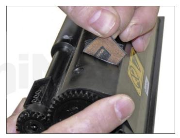
6. Peel off the old chip label (it is an RF type chip).
