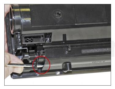
3. If open, close the port by turning a tab on the gear with a screwdriver.
