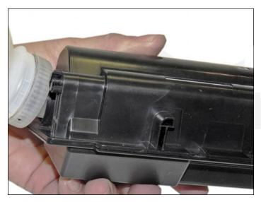
3. Fill the cartridge with toner for use in the TK-17 series of cartridges. Replace the fill plug.
