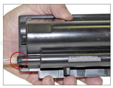
2. Make sure the toner port is closed, by turning the end screw using a slotted screwdriver.
