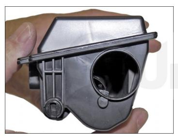
1. Remove the fill plug using a small jeweler's screwdriver.
