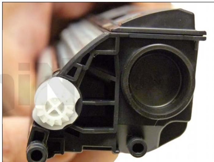
1. Remove the fill plug and dump out any remaining toner.
