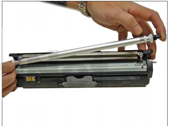
5. Slide the gear side bushing out and remove the mag roller.
