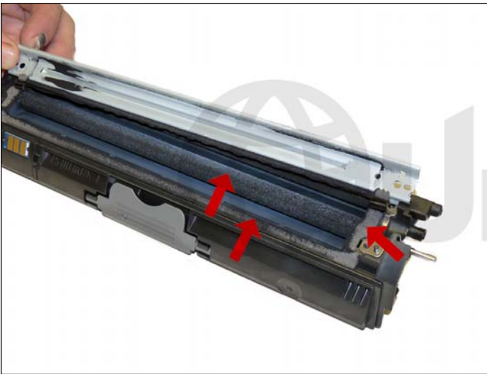
8. Clean out any remaining toner from the hopper, foam seals and the feed roller.
