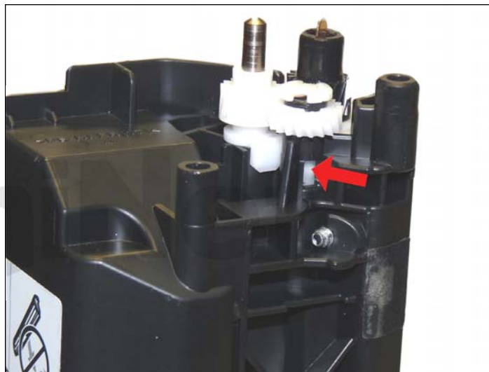
2. On the gear side of the cartridge, pry in on the tab of the gear lock. Remove the lock.
