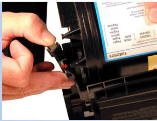
10. With either the small flat head screwdriver or the needle nose pliers, replace both springs on to the Toner Supply Chamber.
