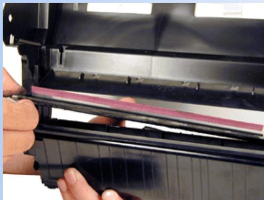
**NOTE 1:** The OEM Wiper Blade has the PCR cleaning assembly attached to it. It cannot be removed from the Blade without damaging it. Our new replacement Wiper Blades come complete with this assembly attached. The first after market Wiper Blades released did not have this cleaner attached. This is OK to use for one cycle, but they should be replaced with a blade that has the cleaning assembly attached.
