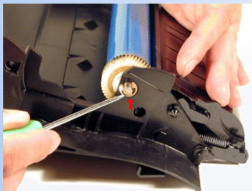
3. Slide the Drum Axle out of the cartridge. Hold the small helical gear while pulling it out so that the drum is not damaged in the process.
