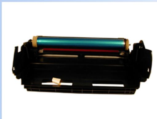
2. Remove the E-Ring from the small helical gear end of the drum axle. There is no need to remove the other E-ring.
