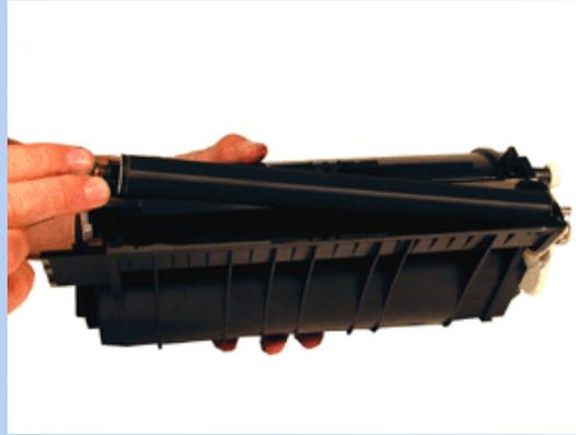
5. Remove the fill plug from the hopper. Pry the plug out from the base next to the hopper. This fill plug is also unique to this cartridge, the fill plug is also a breather cap. It is best to remove both sections at once and to clean them from the outside. These plugs tend to leak if they have been separated.
