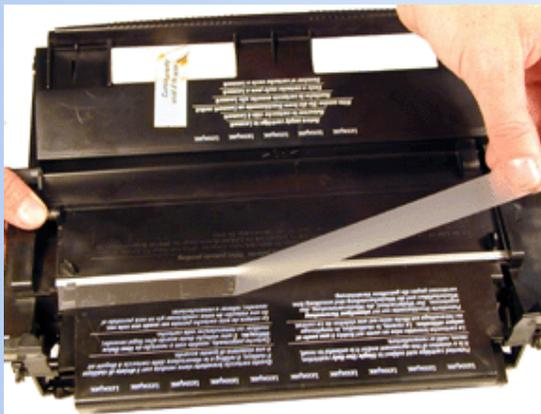
**NOTE:** Be careful not to allow any tape into the laser port opening!
