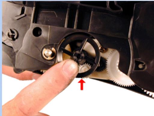
12. A shipping lock must now be installed. This lock should be used even if you are going to hand deliver the cartridge. It will prevent the toner hopper from coming in contact with the OPC Drum, and causing damage to either the Drum or the Static Roller. Press the two red tabs into the sides of the cartridge as indicated in the picture supplied with the lock. When packaging the cartridge, make sure you include a new Felt Wand.
