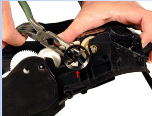
5. Note that there are two posts from the hopper that fit into the cartridge shell. Pull the shell out to release the posts, and lift up the hopper so that the posts are free.
