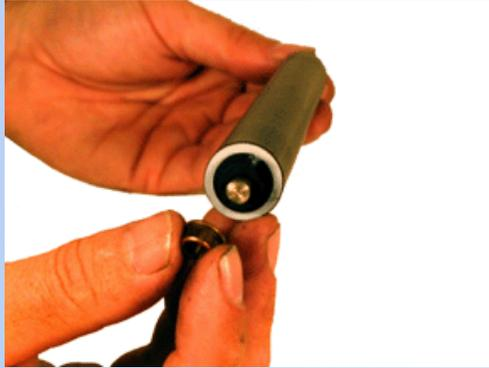
11. Place the keyed end of the Static Roller into the cartridge, and install the roller. Turn the bushing so that the notch is facing down. This will lock the roller in place.
