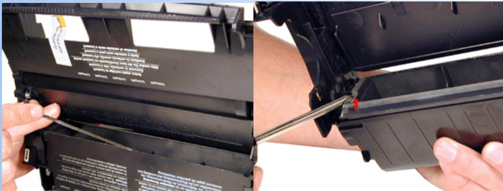
5. Hold the cartridge so that it is up right (Standing up with the waste bin on the table). With one hand, hold the laser shutter open, and with the other hand, remove the Wiper Blade.
