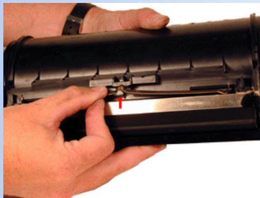
3. On the left side of the Static Roller there is a small bushing, take a small screwdriver, and turn the bushing up so that the notch on the bushing is facing up. This will release the bushing, and Static Roller.
