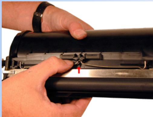
13. Fill the hopper with the appropriate amount of toner. Remember, the amount of toner that can be placed in the cartridge is controlled by the Encoder Wheel. Use 480G for the 17.6k cartridge, and 250g for the 7.5k cartridge. Install the Fill Plug.
