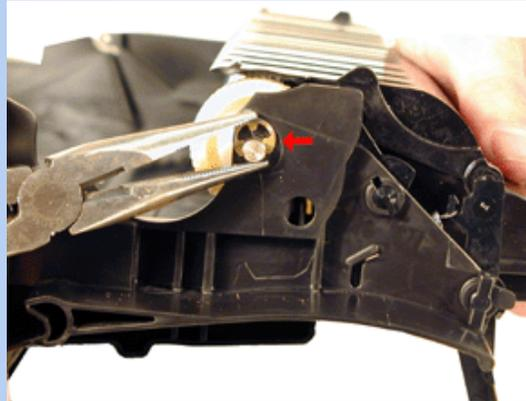
7. Spin the drum for a few revolutions towards the drum cover to ensure the drum and wiper blade are properly lubricated.
