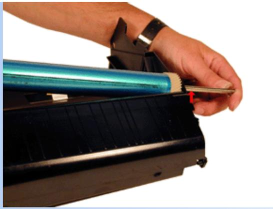
4. Gently lift the Drum and Drum washer up and out of the cartridge, and place in a light protected area. Be careful not to lose the spring and two washers from the large drum gear if present. Not all cartridges have this spring, if it was present, make sure you replace it, if not don't worry about it. It's purpose is to keep the drum from rotating backwards.
