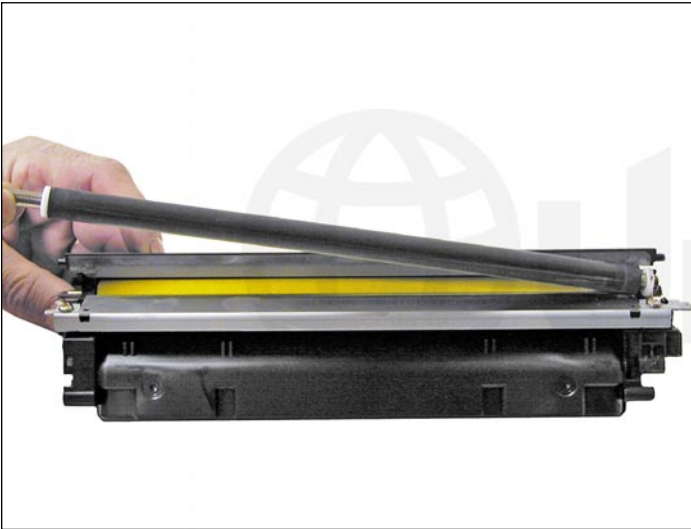
12. Slide the developer roller over, and remove.
