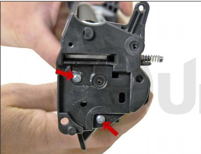
25. Install two small screws into the holes previously drilled out. Leave the top third hole alone (this weld was broken when the end cap was removed). A screw here will interfere with installing the cartridge in the printer. In our tests, the two screws will hold the end cap on with no problems.
