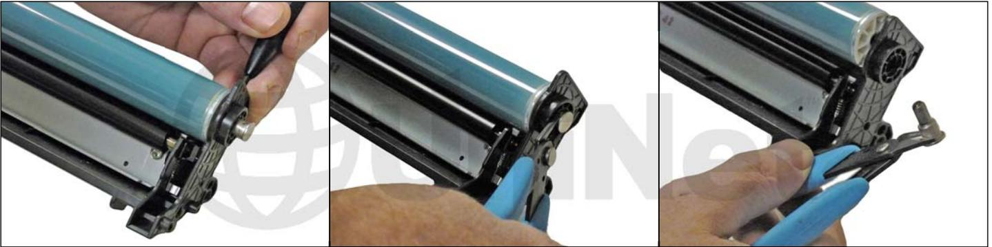
5. With a flat head screwdriver, press the drum axle pin out from the inside of the cartridge wall as shown. There is a small shoulder visible that the screwdriver should be pressed against. Make sure not to bend or damage the plastic wall and the plastic is thin and easily damaged. Remove the axle pin from the outside with flush cutting wire cutters.
