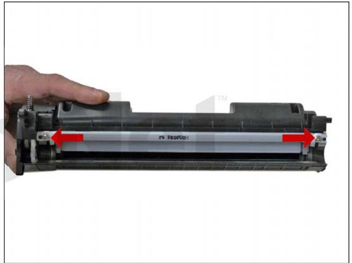
17. Remove the doctor blade and two screws.
