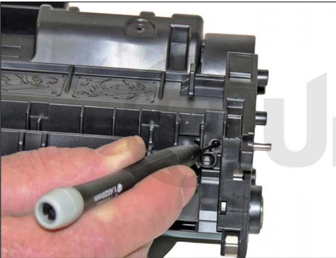
3. Push the pins out with a jeweler's screwdriver. With the hole in this location by just pushing the screwdriver in, the pins will be pushed out. Remove the pins.
