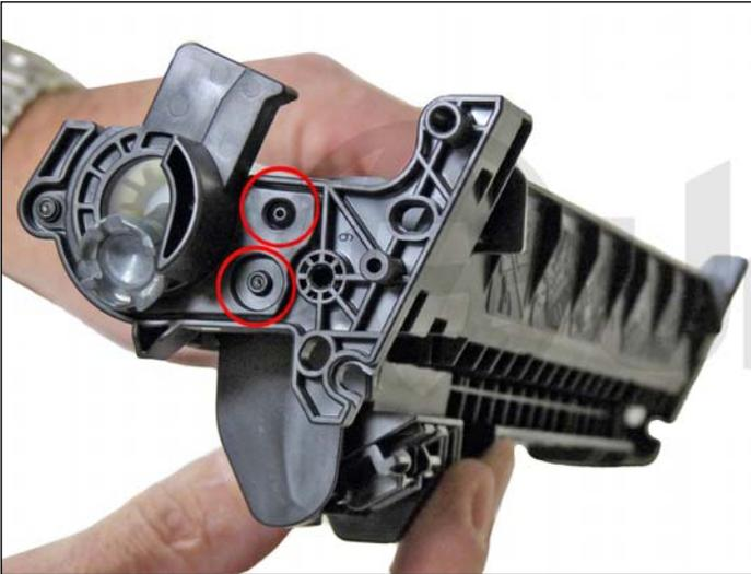
The drum hub on the opposite side is welded. The weld can be broken or drilled out, but there is a good chance that the hub will either warp if pried off, or will be hard to align if drilled out.
