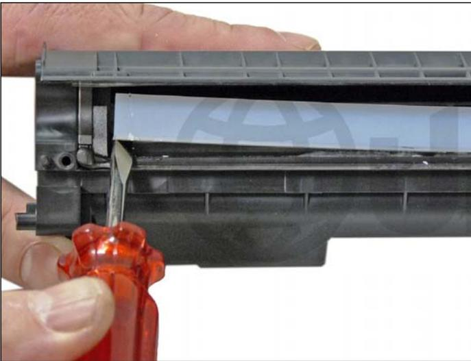
20. If you are going to seal the cartridge, there is a white plastic shelf that needs to be removed. The shelf is held on with double sided tape. It can be gently pried off with a small screwdriver.
