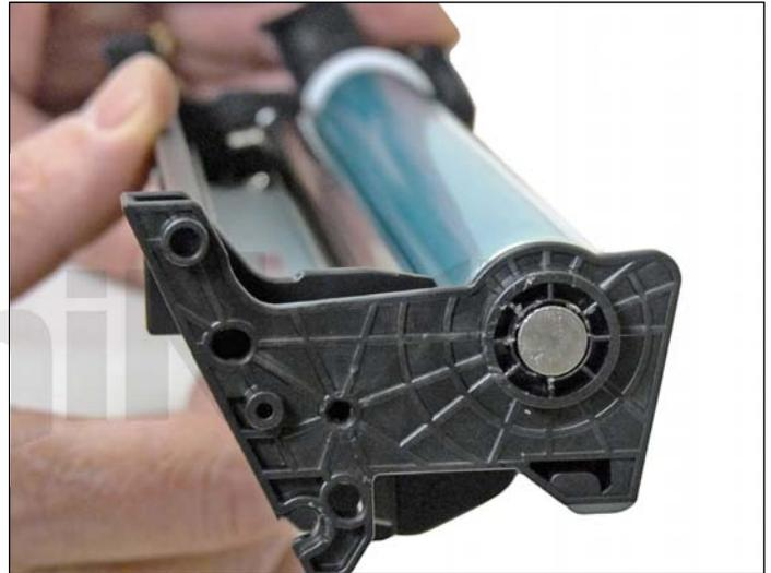
11. Re-Install the OPC drum and metal axle pin. The metal axle pin should have a small amount of conductive grease on the tip.
