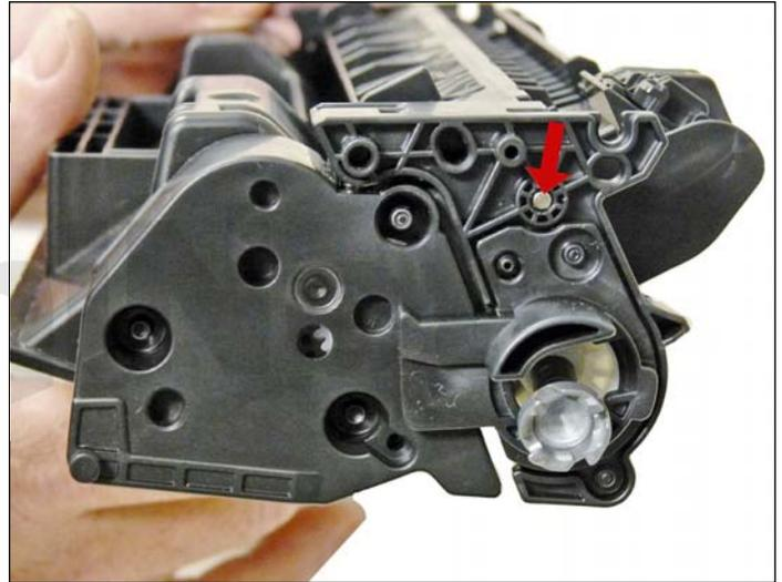
26. Place the two halves together, make sure that the two springs are aligned, and insert the two pins.
