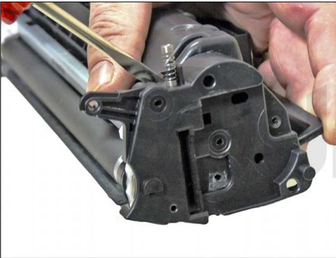
14. With a flat head screwdriver work the edge of the blade around the edge of the end cap and gently pry up the end cap. You will hear the remaining parts of the welds break free. The top weld will also break off now. Take your time with this.
