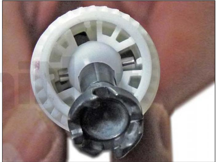
6. Remove the drum. This is a good time to look at the new drive gear(s). This is a completely new system. New drums and gears are being developed.
