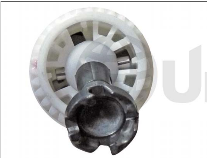
1. Swivel hub on the OPC drive gear shown.
