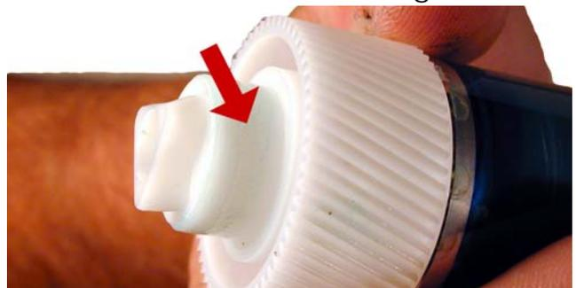
13) Install the spring in the holder as shown, install on the cartridge and set the tail of the spring so it drops into its slot. See **Figures 27 & 28**
